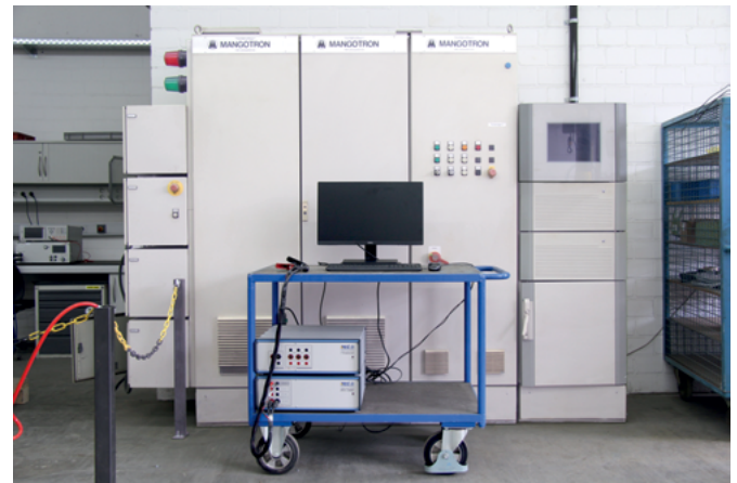
Figure 5: Control cabinets of the DC linearity test bench in the background, in front trolley with DPG10-4000B/F and PC
