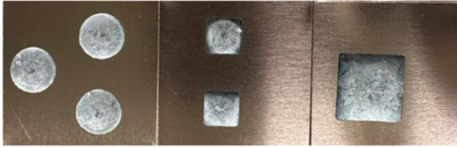
Figure 9: Reflow Results for High-Pb Fluxless Solder Paste - Component-Attach
