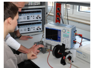
Figure 5: Using a 1000 A pulse current source, the time delay through the transducer is measured.
