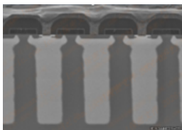
Figure 8: SEM image of Sanan's Superjunction Mosfet (platform in development) reaching below 1.5 mΩ*cm2 for a 1200V device
