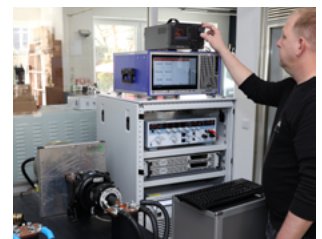
Figure 6: At the high-power test bench, DC power and AC low-frequency power with variable power factor can be simulated up to 1200 V and 2000 A.
