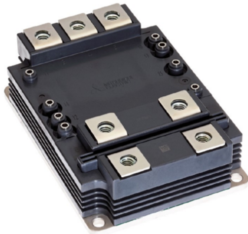
Figure 11: The LV100 package for the FMF1600DC-50CW and FMF800DC-66BEW.
