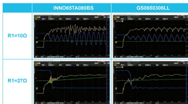
Figure 4: Measured waveforms at 10\Omega and 27\Omega
