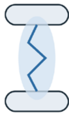
Figure 2: Contact erosion. A molten bridge transfers metal as the contacts part, the arc melts and vaporises more, and over many operations a pip and crater form while the surface oxidises.
