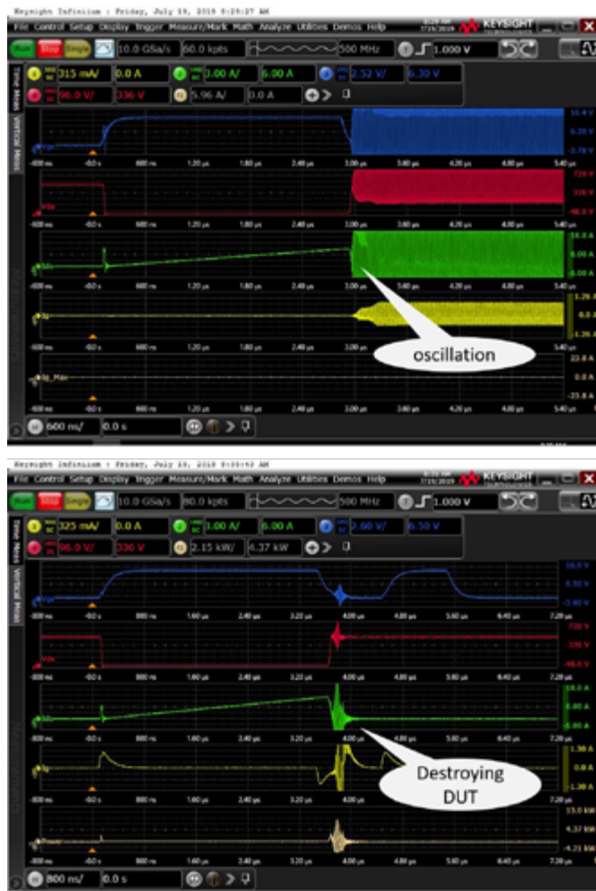
Figure 1: GaN FET double pulse test results with oscillation.
