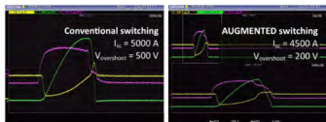
Figure 7: Demonstration of how augmented switching (right) can reduce peak voltage and peak current during short circuit event compared to conventional switching (left)
