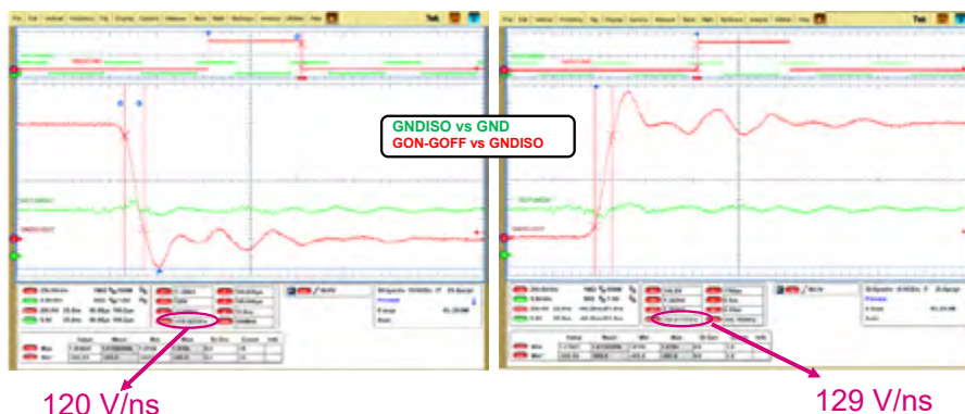
Figure 1: Measured positive and negative transients in the STGAP2S, V_{DC}=1500 V.
