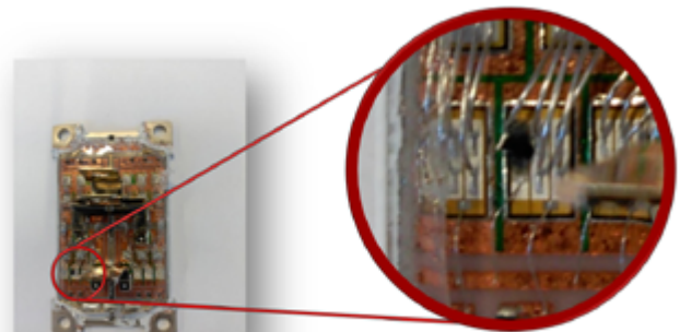
Figure 8: Post-failure analysis on a commercial SiC MOSFET module after a short circuit test, showing a burnt spot on a chip.
