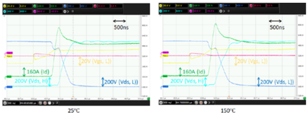
Figure 5: IGBT power module test result examples (25 °C & 150 °C).
