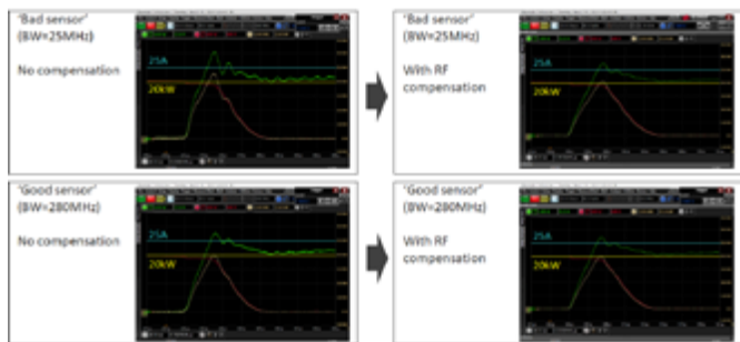
Figure 2: Effect of RF compensation on drain current.
