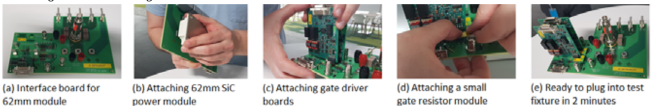
Figure 4: DUT interface board and gate resistor module.
