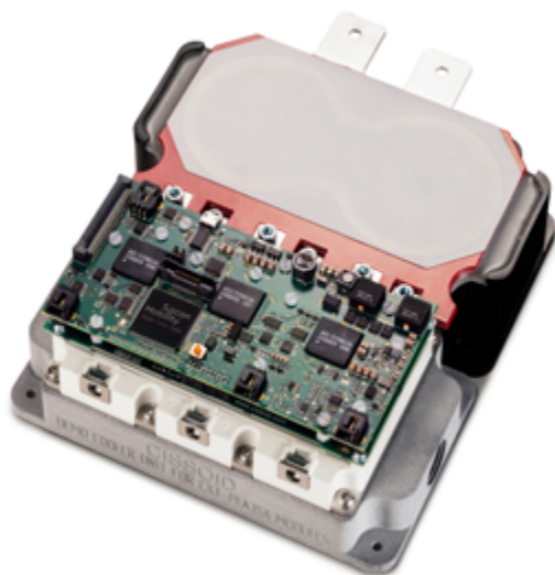
Figure 1: Cissoid's SiC Inverter platform.
