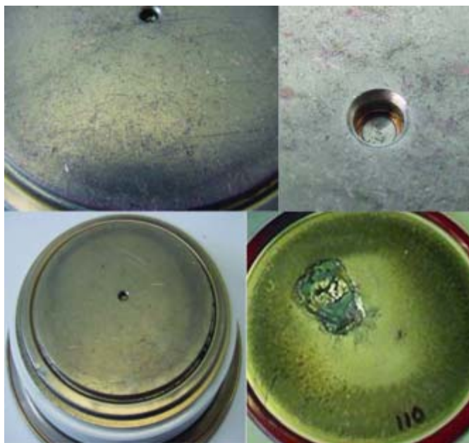
Figure 2: Failure Due to Mounting Error Exhibits Silicon Melt on Cathode
