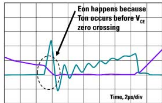
Detail of IGBT's IC & VCE
