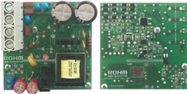
Figure 4: Evaluation board for SiC based auxiliary power supply unit
