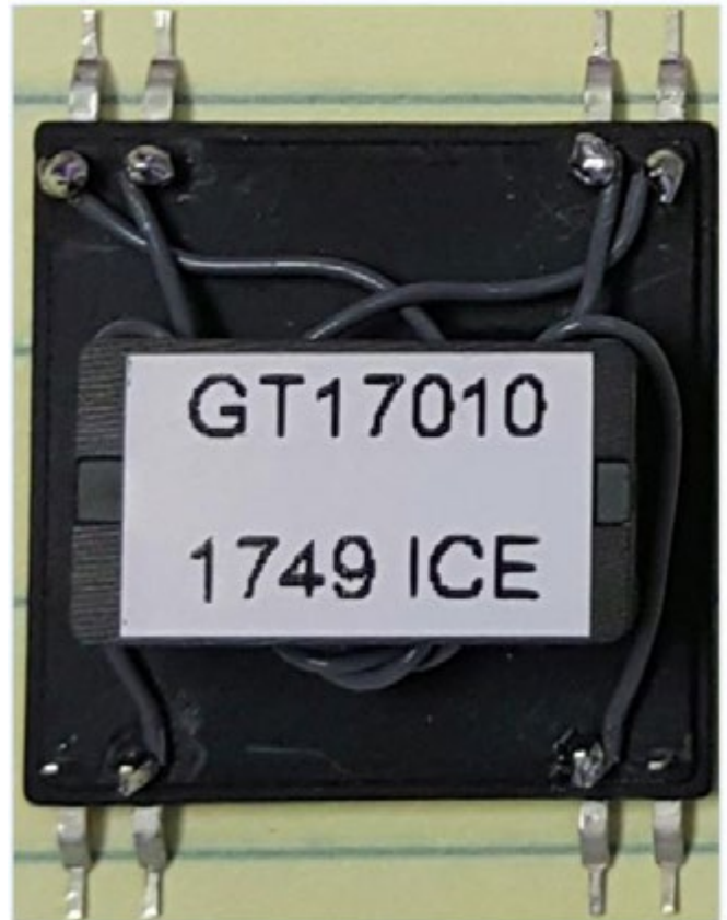
Figure 2: Prototype with top of core removed to show the trifilar windings
