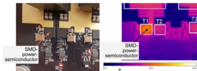
Figure 3: PCB and thermal measurement of the PCB based multilevel converter at 1 kW per Phase
