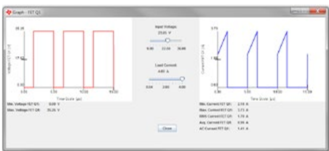
Figure 2: Graph window for the FET Q1 in a flyback converter displaying waveforms for voltage and current
