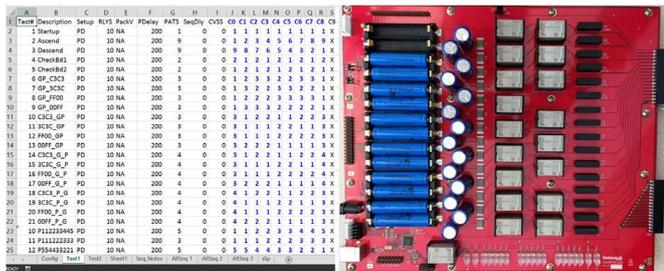
Figure 3: Hot plug tests consist of switched connection sequences
