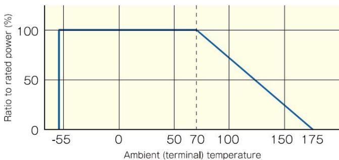
Figure 2: Indicating power rating at  $70^\circ\text{C}$
