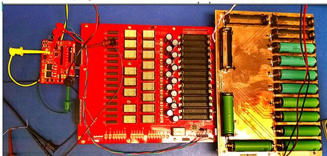
Figure 1: A hot plug test requires programmable switching for control/timing of each cell connection
