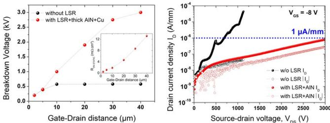
Figure 8: Evolution of LGD-dependent device breakdown and specific on-resistance (inset) of AlGaIn/GaN HEMTs with and without LSR/thick AlN/Cu by defining the blocking voltage at 1  $\mu\text{A}/\text{mm}$ , and off-state leakage current characteristics of AlGaIn/GaN MISHEMTs with and without LSR / thick AlN deposition.
