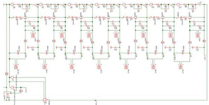
Figure 4: View of BMS hot plug connections from an overall circuit stress viewpoint
