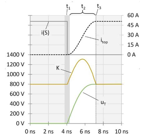
Figure 2: ZOS Switching wave form
