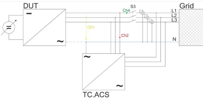
Figure 3: Test set-up using TC.ACS Impedance Simulation. For voltage and frequency related tests switch S3 stays open and the grid is being simulated by TC.ACS operated in Grid Simulator mode. For the detection of islanding switch S3 is closed, TC.ACS is operated in R-L-C-Simulation mode and the simulated R-L-C-circuits are adjusted in full operation. S3 is reopened again to test the DUT’s behavior while in islanding condition.
