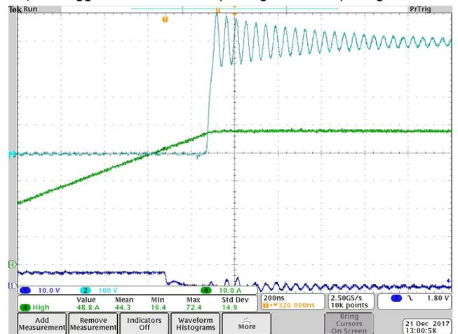
Figure 5: Turning off a non optimal current
