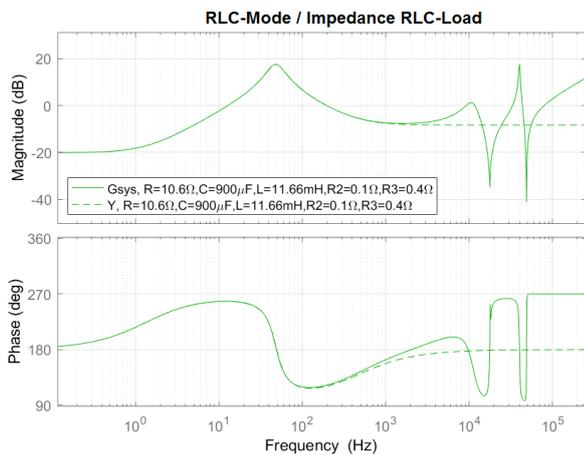
Figure 8: Comparison of the simulated (continuous) and the real (dotted) impedance according to the topology 12 of the RLC-operation with the following values:  $R=10.6\Omega$ ,  $C=900\mu F$ ,  $L=11.66mH$ ,  $R2=0.1\Omega$ ,  $R3=0.4\Omega$ . The influence of the TC.ACS output filter is clearly visible in the Wfrequency range  $> 1kHz$ .
