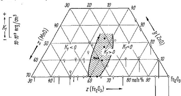
Figure 3: K<sub>1</sub> vs MnZn composition diagram
