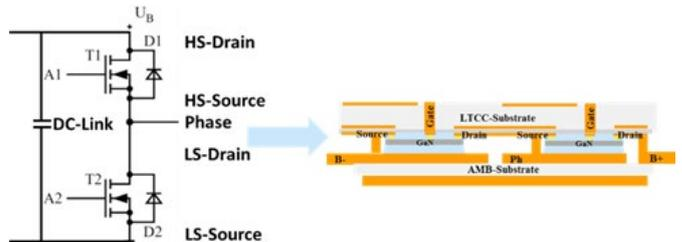
Figure 9: Rough sketch about the transition from half-bridge topology to power module design.
