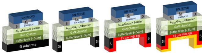
Figure 6: Schematic cross-section of AlGaIn/GaN MISHEMT after the front side process, the LSR technique, 15  $\mu\text{m}$  thick PVD AlN deposition, and the 2  $\mu\text{m}$  Cu deposition on the back-side.
