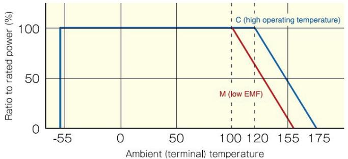
Figure 3: Curve shows higher derating point
