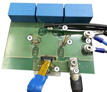
Figure 4: ZOS test platform with module-integrated gate drivers, increased link inductance and film capacitors
