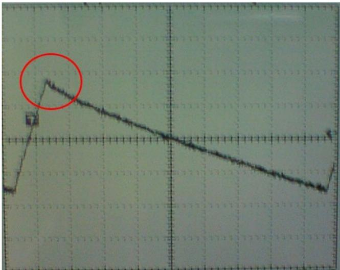
Figure 5: The same waves when using a long-side terminal resistor, demonstrating a clear reduction of the switching noise
