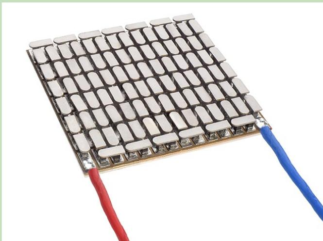
Figure 1: About 60 to 70 grams of half-Heusler material are installed in a thermoelectric generator (in the image) to convert waste heat into electricity.
