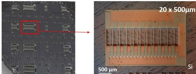
Figure 7: Optical backside image of the wafer with and without LSR removal patterns, and a  $20 \times 500 \mu\text{m}$  GaN-based MISHEMT after LSR.
