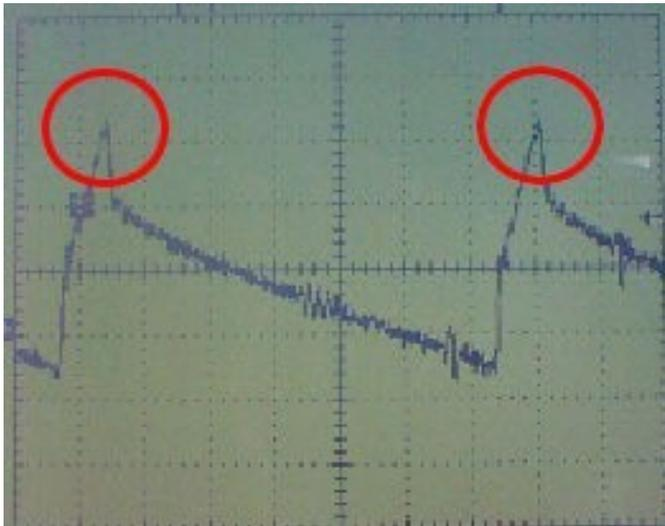
Figure 4: The shape of the waves using a short-side terminal resistor with the switching noise
