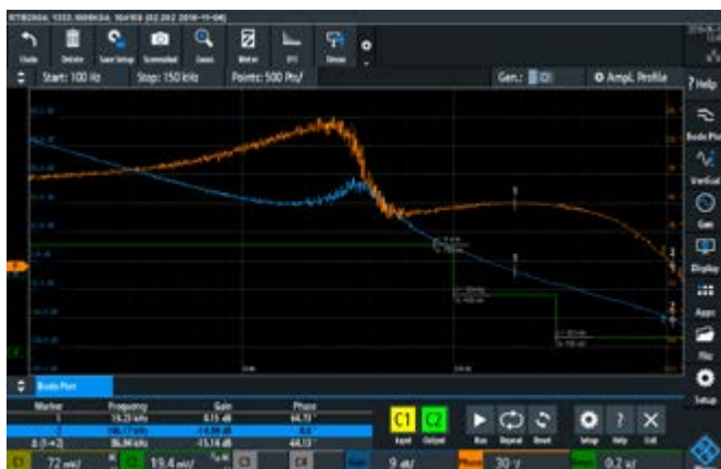
Figure 3: Optimized amplitude profile of the injection signal (blue) and bode plot (red and blue)
