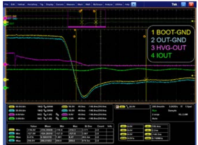
Figure 3: 127 \text{ V} Below-ground observed on channel 1 output with a stray inductance of 0.82 \mu\text{H} .
