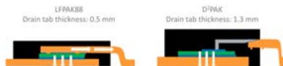
Figure 5: D 2 PAK and LFPAK88 thinner drain tab
