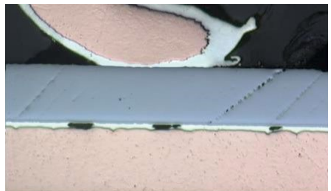
Figure 6: Cross-section of an AlCu bond wire
