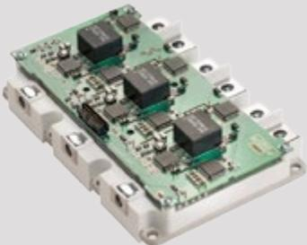
Water-cooled 3-Phase 1200V/600A SiC MOSFET Intelligent Power Module
