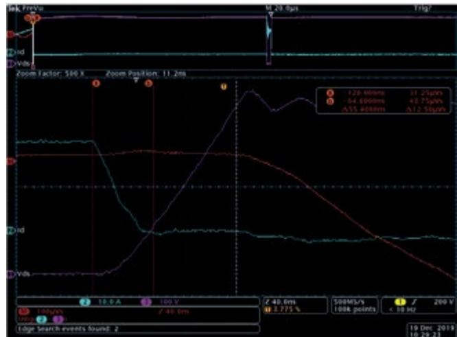
Figure 5: Pre-Switched turn-Off wave form of 1200V 35mOhm MOSFET (United SiC UJ3C120040K3s) at 800V and 40A. Note the non-overlapping current (blue) and voltage (purple) wave forms and virtually no switching losses (red).
