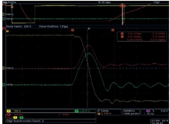
Figure 3: Pre-Switched ARCP turn-On waveform of 1200V 35mOhm MOSFET (United SiC UJ3C120040K3s) at 800V and 40A. Resonant current (green), voltage (yellow), ARCP loss (red).
