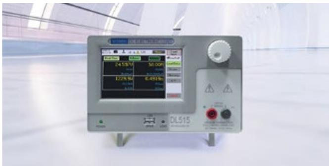
250W and 500W), each with input voltages of 0-150V or 0-500 VDC. Unlike comparable programmable DC loads, the DL Series is capable of supporting loading sequences utilizing constant voltage (CV), constant resistance (CR), constant current (CC) and constant power (CW) in any combination in single or arbitrary sequences of up to 100 steps.
