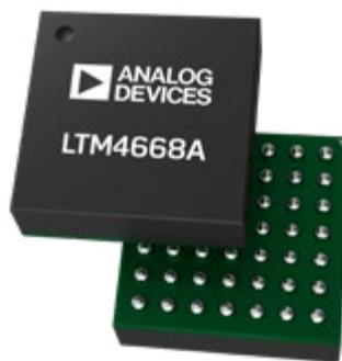
Operating over an input voltage range of 2.7V to 17V, the LTM4668 and LTM4668A support an output voltage range of 0.6V to 5.5V. The devices support frequency synchronization, PolyPhase operation, selectable Burst Mode operation, 100% duty cycle and low IQ operation. Their high switching frequency and a current mode architecture enable a very fast transient
