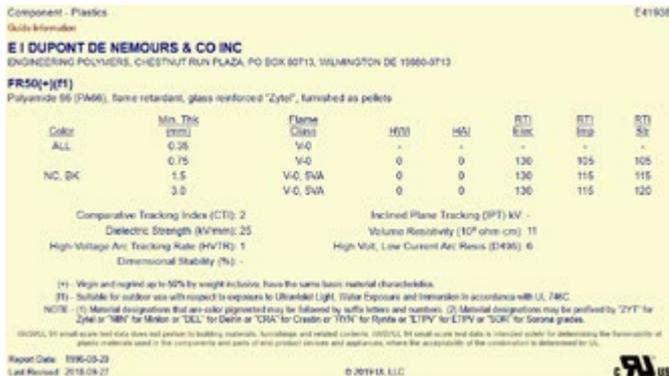
Figure 2: Example of the UL "Yellow Card" for FR50 PA66 plastic material
