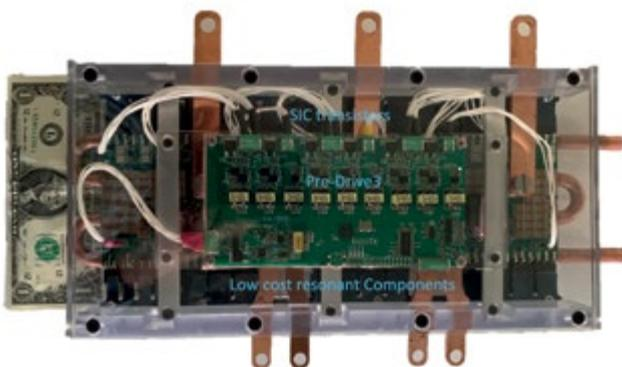
Figure 7: CleanWave200 evaluation system (200kW inverter power block, 800Vdc, 99% efficiency at 100kHz).
