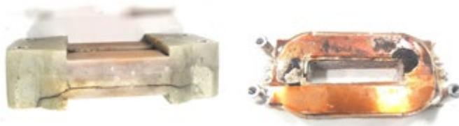
Figure 1: Excess of heat can lead to electrical breakdown of power components
