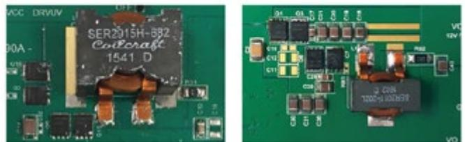
**Figure 2:** Size comparison of a nonisolated buck converter and equivalent 48 V to 12 V/20 A hybrid converter.
