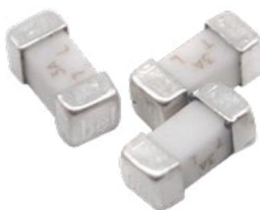
Bel's 0680L Series fuses are compatible with the 260<sup>°</sup>, IR Pb-free solder process and feature a current rating from 375mA to 12A and a wide operating temperature range of -55<sup>°</sup> to 125<sup>°</sup>C. These fuses are also AEC-Q200 compliant, RoHS compliant (with exemption 7(a)), halogen free (MSL = 1)
