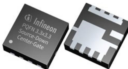
footprint is based on the current PQFN 3.3x3.3 mm pinout configuration. The location of the electrical connection remains the same, simplifying the drop-in replacement of today's standard Drain-Down packages with the new Source-Down package. For the Center-Gate version, the gate-pin is moved to the center supporting easy parallel configuration of multiple MOSFETs.
