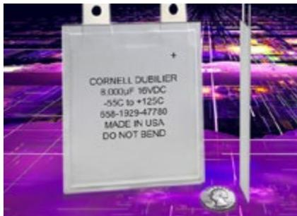
tors. Custom values are available within a capacitance range of 8,000  $\mu\text{F}$  to 20,000  $\mu\text{F}$ , with working voltages ranging from 6.3 to 24 WVDC. The company plans to extend the series to higher operating voltages later in the year. Operating life is 2,000 hours @ 125° C. The PPC is rated for 10 g peak for vibration and withstands shocks up to 100 g's (MIL-STD-202, Method 213, Condition I).
