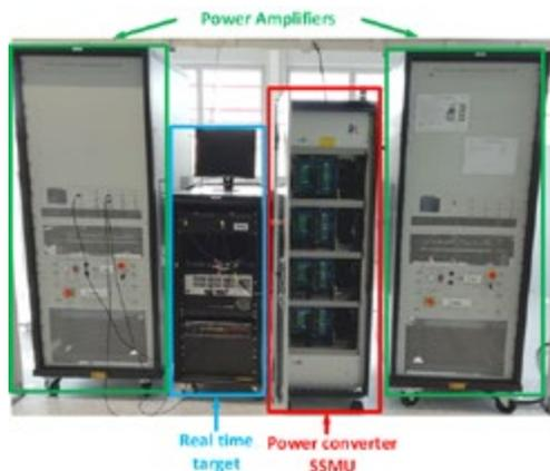
Figure 4: Experimental PHIL test bench
