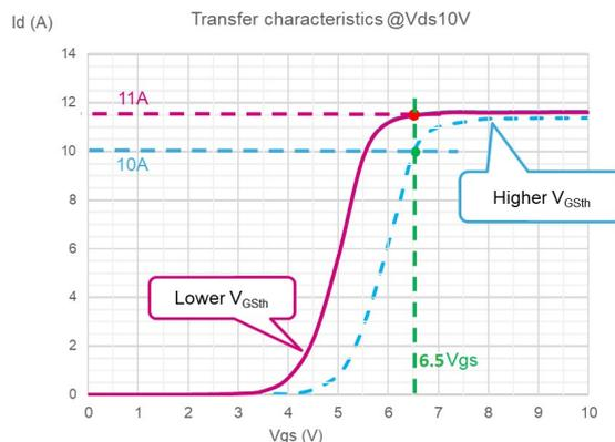
Figure 5: Transfer characteristics for MDmesh™ technology, in purple with V<sub>GSth</sub> = 3V and in dot blue with V<sub>GSth</sub> = 4V
