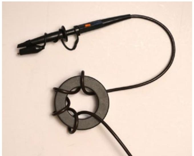
Figure 5: Voltage probe with some added common mode impedance
