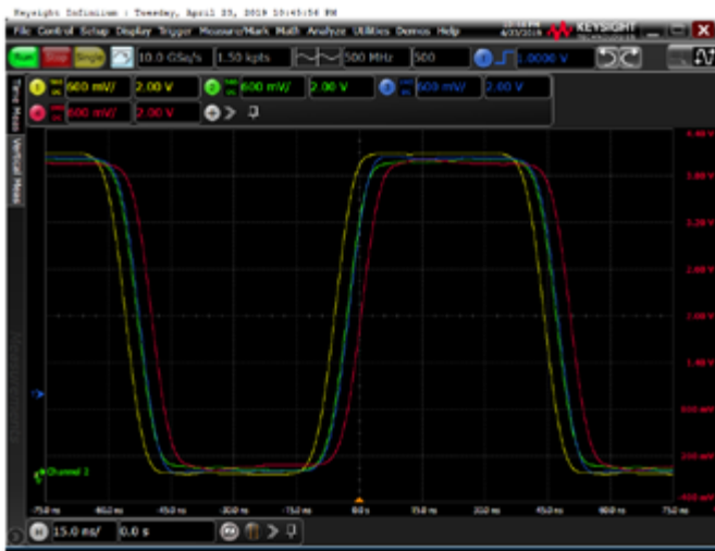
Figure 6: Time skew in oscilloscope inputs, measured on DPT fixture
