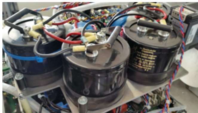
Figure 3: The GW series capacitors are used by Schumacher for example in the power supply units for high-power laser diodes in research systems
