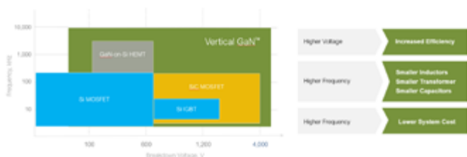
Figure 2: Vertical GaN™: A Superset of existing Power Semiconductor Technologies
