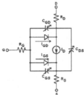
Figure 7.15: Elements of a SiC jfet. The arrows indicate that all capacitances shown are voltage-dependent  $V^{-1/2}$ . Like all fets these have a  $TC = 0$  point where the increase of the on-resistance with temperature matches the negative gate voltage characteristic of  $-2.3$  mV/degree.
