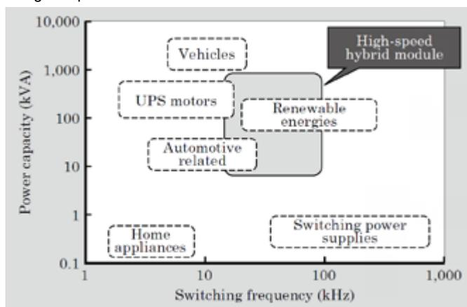
Figure 1: Main applications of high-speed hybrid modules
