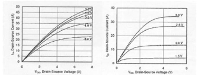
Figure 7.14: Characteristics of Semisouth jfets (left) and their so-called "enhancement" jfet, a great flop and possibly the reason for folding up.
