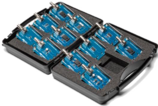
Figure 12: Full set of evaluation boards for SiC CLD assessment.
