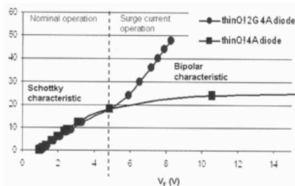
Figure 7.9: The characteristics of "pure" and 2nd generation SiC diodes show the takeover of the current by the parallel pn diode, protecting the former.
