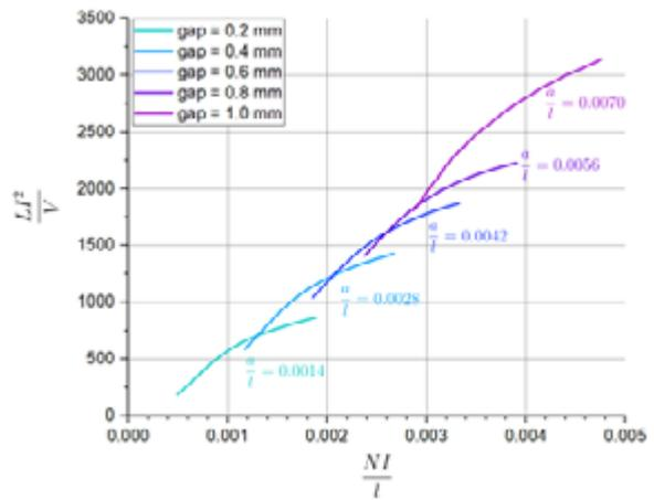
Figure 8: Hanna Curve of D9B in EE65 core with different gap length (in SI).
