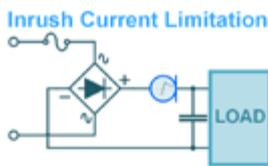
**Protection of Sensitive Equipment from Transients Generated by Switching of Heavy Loads**
