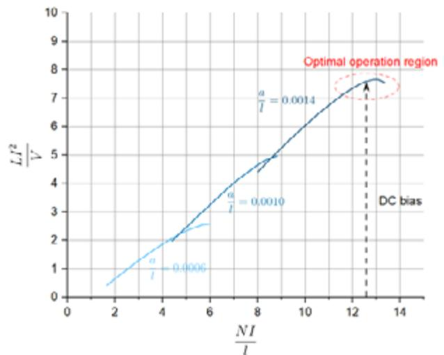
Figure 4: Typical Hanna Curve of a gapped core.
