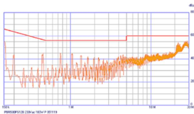
Figure 3: AC-DC power supply, internal filter only
