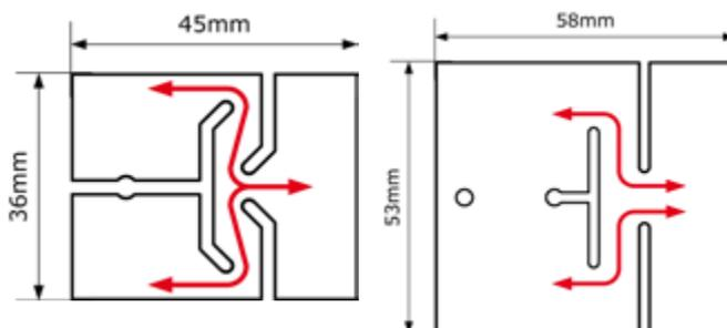
Figure 2: PCBs with creepage distance
