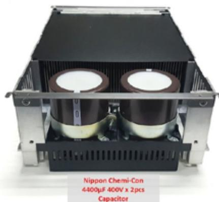
Figure 3: The DC bus capacitor.
