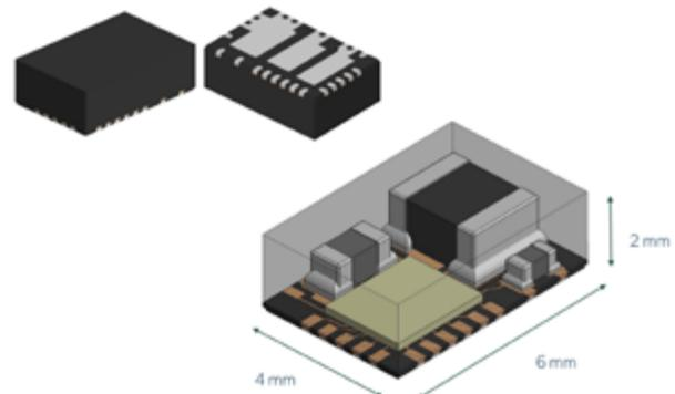
Figure 1: The APM80900 is a 40 V, 1.5 A synchronous buck LED driver ClearPower module by Allegro MicroSystems
