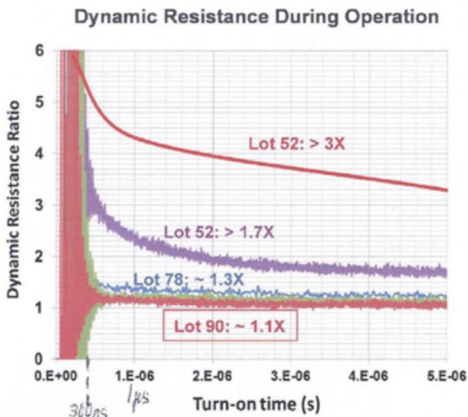
Figure 8.4: Dynamic on-resistance of GaN transistors (RFMD). The picture shows a strong dependence on the lots. The decay to the static value requires microseconds i.e. times far above the switching times. The picture further shows that the increase is far above a 6-fold one where the vertical scale ends.
