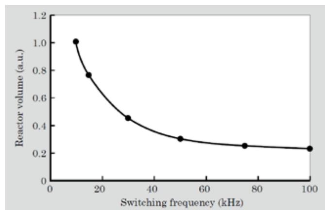
Figure 3: Dependence of reactor volume on switching frequency
