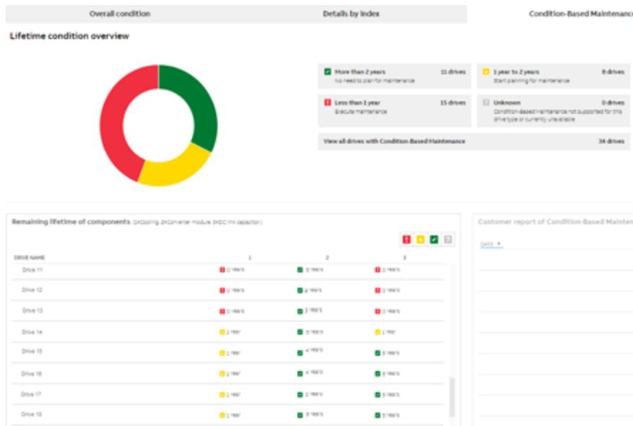
Figure 4: The dashboard provides an immediate overview of the maintenance needs of the complete fleet of drives.
