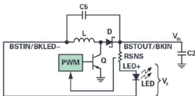
Figure 3: LTM8042 block diagram connections in buck configuration.
