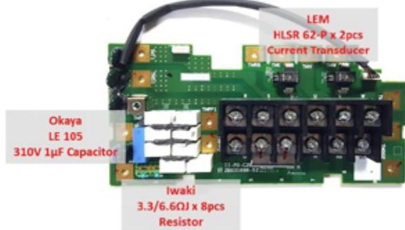
Figure 5: Line input and three-phase output contactor board.
