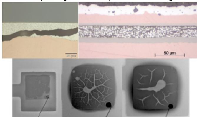
*Figure 1: Modes of failure of silver sintered interconnects, via pressure-less sintering. Top left: crack through the layer, with delamination of the substrate.; Top right: High porosity of sintered silver layer.; Bottom: Drying channels, large voids, delamination.*
