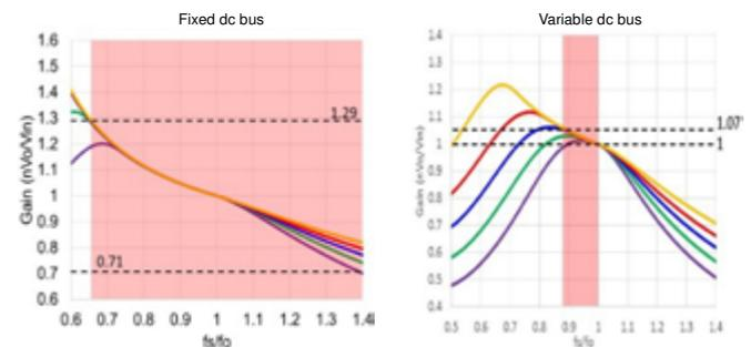
Figure 2.4: Gain curves for fixed dc bus and variable dc bus CLLLC
