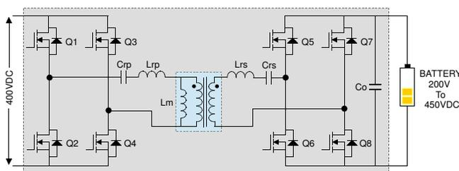
Figure 2.3: CLLLC converter power stage
