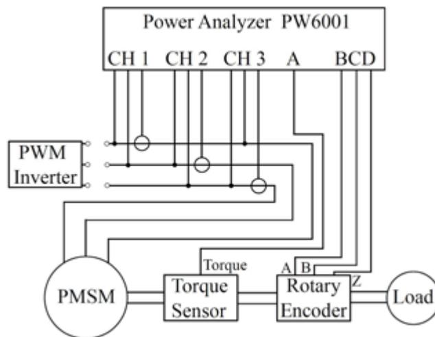
Figure 5: Wiring for phase zero-adjustment and induced voltage constant *Ke* identification.
