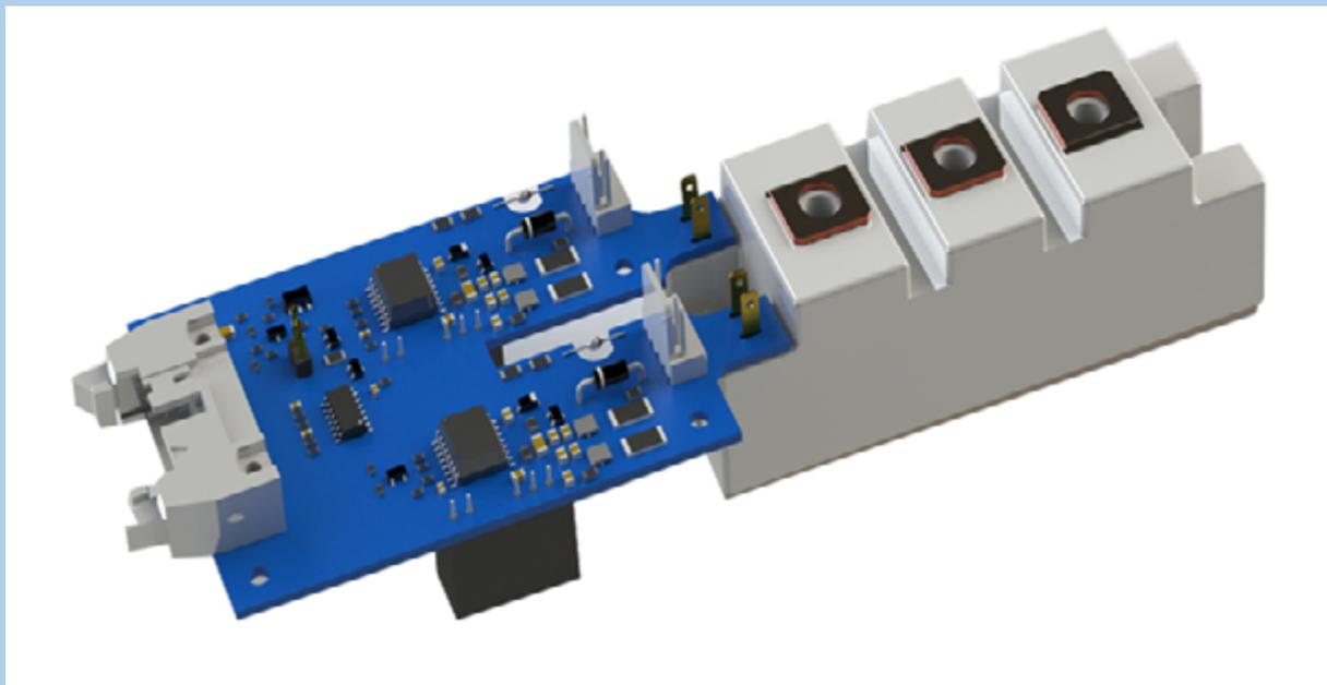
Proton-Electrotex now offers compatible drivers for the entire lineup of its IGBT modules. They are advanced dual-channel plug-and-play IGBT drivers for MIAA, MIFA and MIDA-type IGBT modules with collector current up to 600A and voltage class up to 1700 V.
