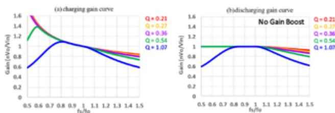
Figure 2.2: LLC charging and discharging mode gain curves
