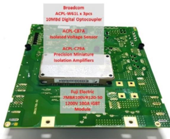
Figure 6: The power electronics board.
