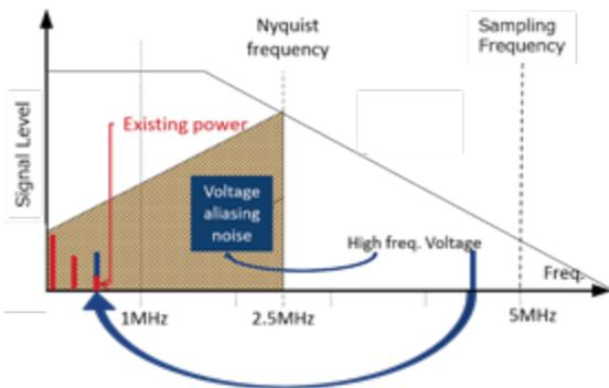
Figure 3(a): Example: 5MHz sampling without AAF
