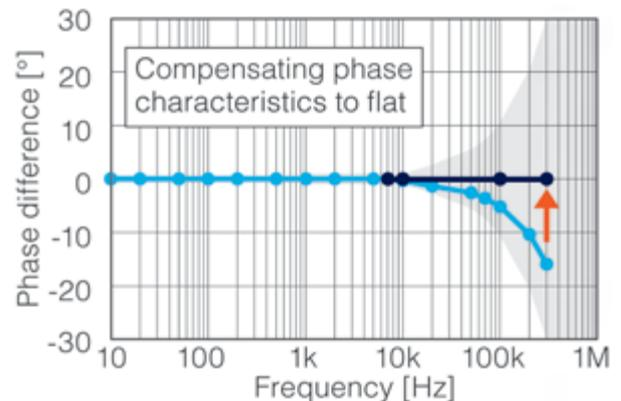
Figure 2: Phase error with and without compensation
