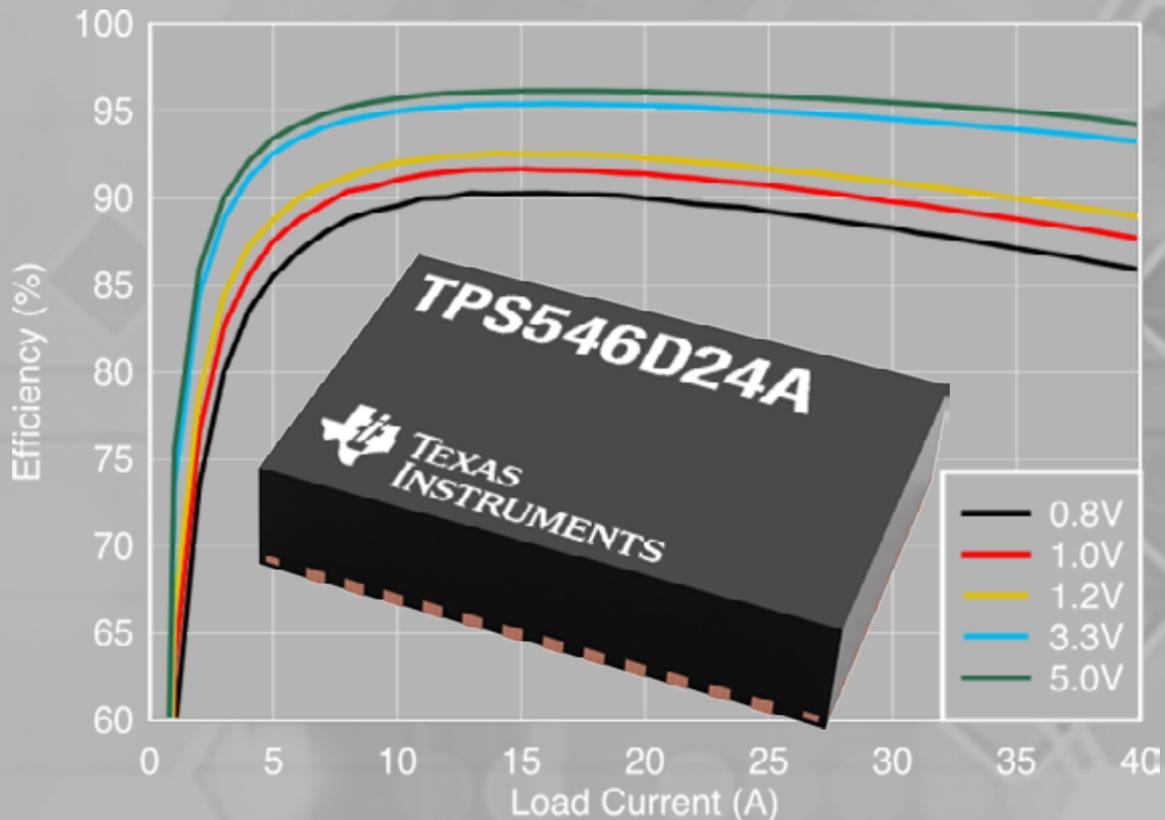
$V_{IN} = 12\text{ V}$                        $L = 300\text{ nH}$
