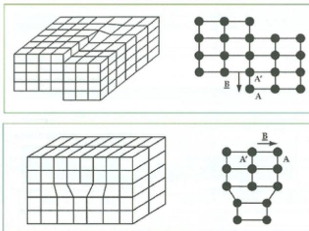
Figure 7.2: Lattice displacements are the cause for the difficulties of producing low-cost SiC semiconductors. A' would be located at A if there were no displacements. There are more lattice defects, all contribute to low yield.
