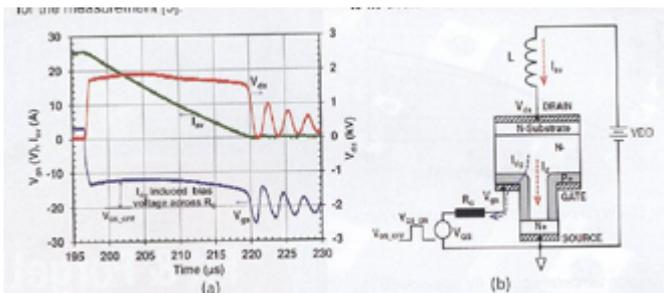
Figure 7.11: Avalanche behaviour of USCI cascodes. The cascode is turned on by the leakage current of the jfet, damping the overload.
