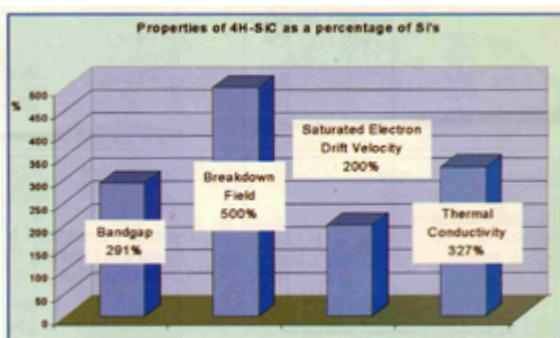
Figure 7.1: Visualization of SiC advantages over silicon.
