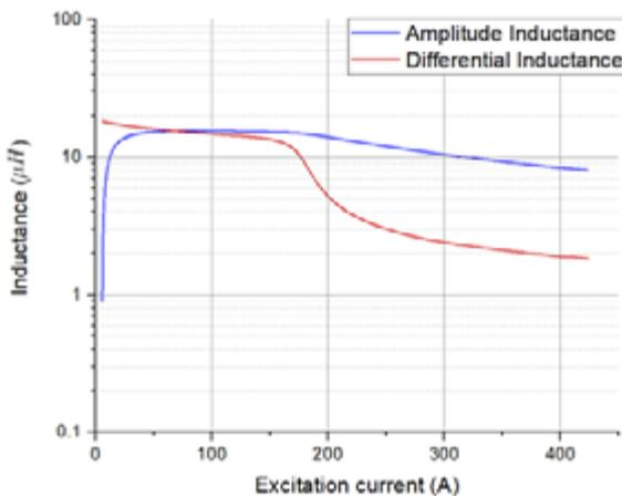
Figure 6: Measurement results for UI 93 ferrite core for leakage inductance with Bs&T pulse.
