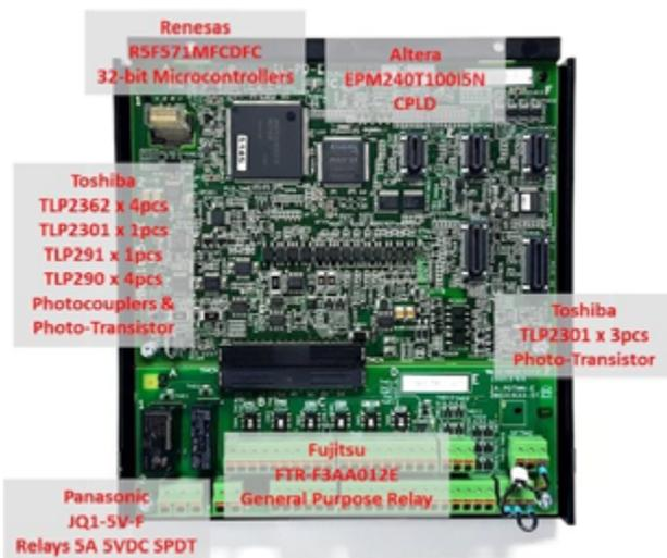
Figure 4: The main controller board.
