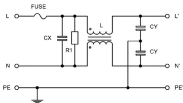
Figure 1: Typical modular EMI filter circuit
