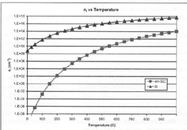
Figure 7.5: Charge carrier concentration of Si and SiC. Apart from the band gap this determines up to which temperatures a semiconductor remains one. This temperature is > 1000 C for SiC. Above the material remains only a resistor.
