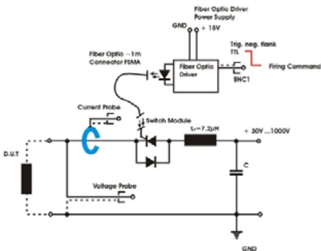
Figure 3: Bs&T measurement system with damped oscillation method.
