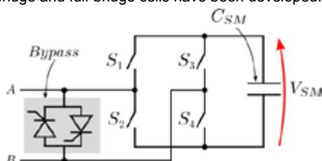
Figure 4: Full-bridge sub-module schematic including the bypass switch.
