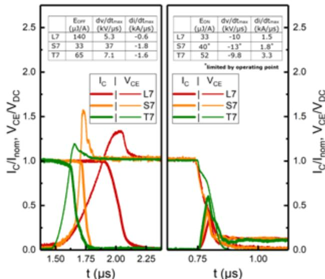
Figure 3: Turn-off waveforms (left-hand side) and turnon waveforms (right-hand side) of L7, S7, and T7 for  $I_C = I_{nom}$  and  $I_C = 0.1 \cdot I_{nom}$ , respectively, with  $V_{DC} = 600$  V at  $T_J = 25^\circ C$ . The tables contain characteristic parameters
