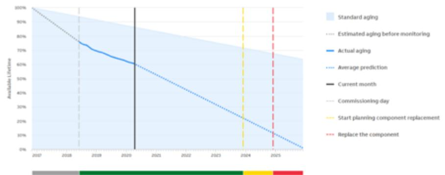
Figure 1: Blue shading indicates the nominal life of a VSD while the blue line shows the predicted life.
