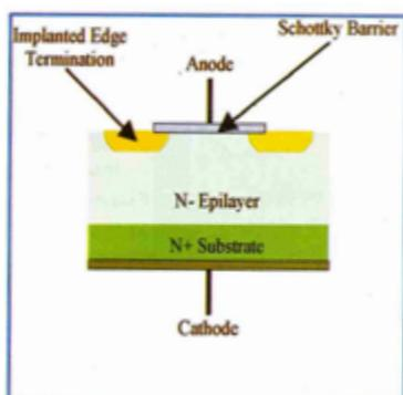
Figure 7.7: Structure of a SiC diode. The diode is constituted by the metal - semiconductor contact, hence it is a Schottky diode with the known advantages. However, the forward voltage is quite high, most diodes are 600 V types with 1.5 V, following the general rule that the forward voltage rises with the blocking voltage.
