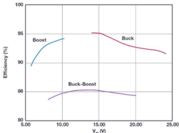
Figure 5: LTM8042 efficiency for boost, buck, and buck-boost configurations.
