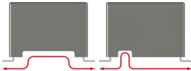
Figure 3: Additional gaps that incorporate the extra creepage
