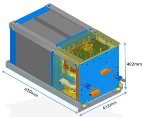
Figure 2: CAD Model of the full bridge sub-module.
