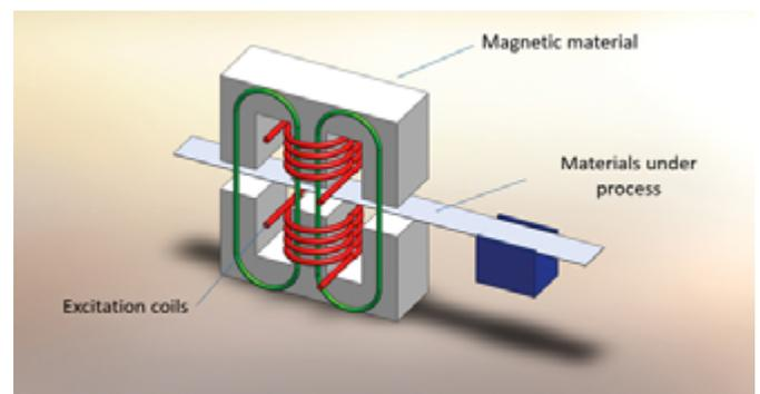
Figure 2: Principle of cross field heating – an application of inductive components working with high temperature and high excitation current.
