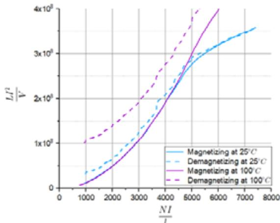
Figure 9: Hanna Curve of D9B in EE65 core with different temperature and magnetizing/demagnetizing process (in SI).
