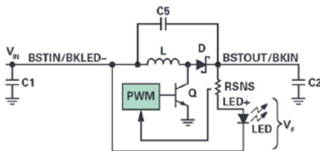
Figure 4: LTM8042 block diagram connections in buck-boost configuration.
