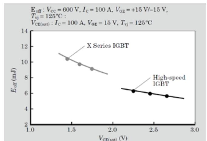
Figure 2: 1200V high-speed IGBT  $V_{ce(sat)}$  -  $E_{off}$  characteristics
