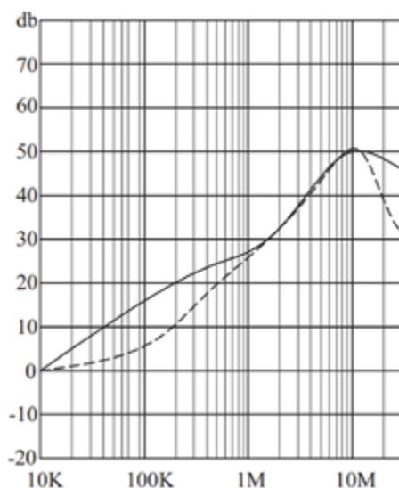
Figure 4: Modular filter type XP FCSS06SFR
