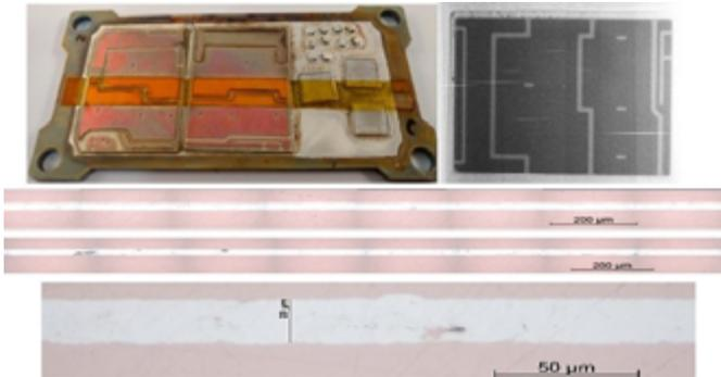
Figure 3: Performance of silver sintered copper-to-copper interconnects. Top left: Demonstrator with a total surface area of 3000 mm<sup>2</sup>; Top right: X-ray scan of one DBC to Cu-plate interconnect; Bottom: Cross section through two copper plates sintered in a pressure-less process with a surface area of 500 mm<sup>2</sup>.
