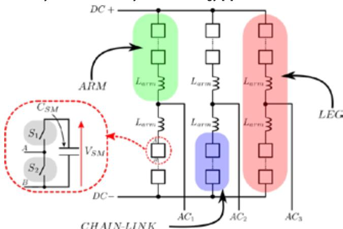
Figure 1: Three phase MMC schematic.
