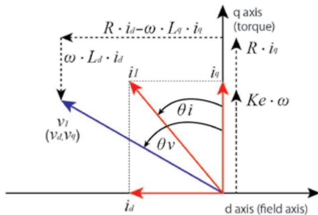
Figure 4: PMSM Vector Diagram
