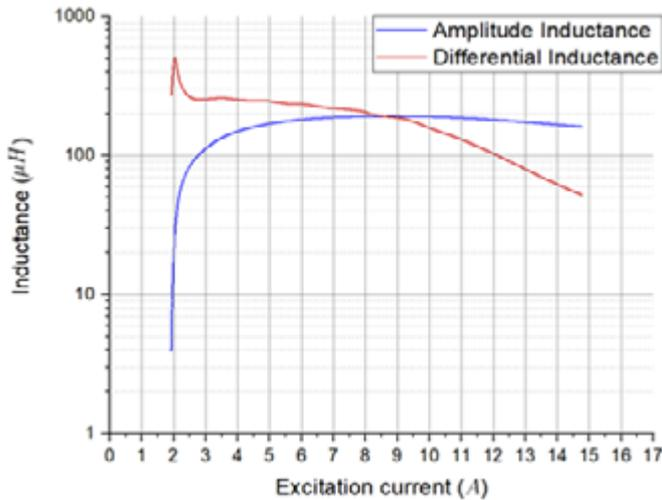
Figure 5: Measurement results for UI 93 ferrite core with Bs&T pulse.
