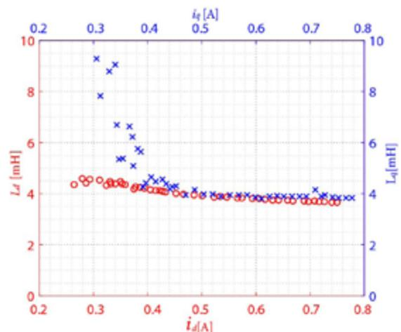
Figure 7: Relationship between the d-q axis current and the identified d-q axis self-inductance
