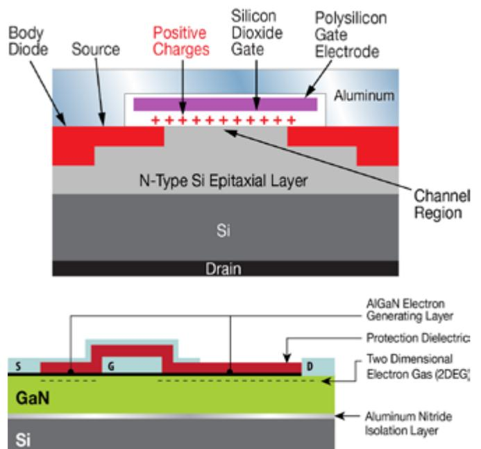
Figure 1: (a) Cross section of a typical silicon MOSFET (b) Cross section of a typical enhancement mode GaN (eGaN<sup>®</sup>) device
