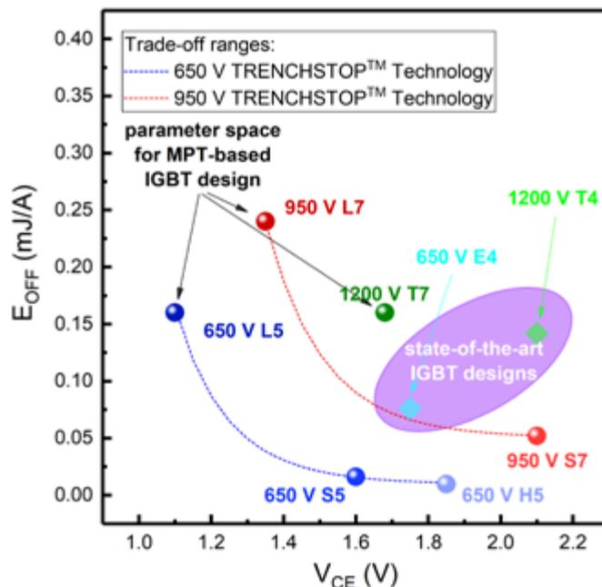
Figure 2: Trade-off diagram of 650 V, 950 V, and 1200 V MPT IGBT technologies. Static and dynamic values are provided at  $T_j=150^\circ\text{C}$  and with  $V_{DC}=2/3 \cdot V_{CES}$ . As a reference, 650 V and 1200 V state-of-the-art, 4th generation IGBTs are indicated as well
