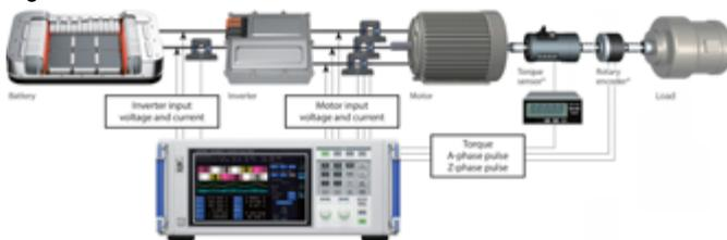
Figure 1: Evaluation system for motor control efficiency with Power Analyzer PW6001
