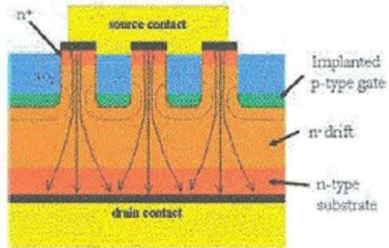
Figure 7.12: Structure of Semisouth jfets. It is purely vertical, the current flows from the bottom contact to the drain and through the drift zone to the source. The gate is covered with SiO<sub>2</sub> in the valleys.
