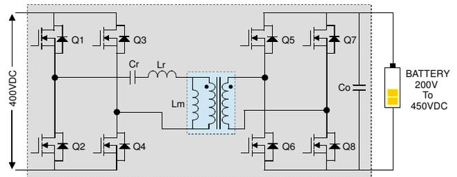
Figure 2.1: LLC converter power stage
