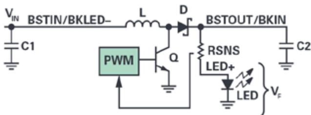
Figure 2: LTM8042 block diagram connections in boost configuration.
