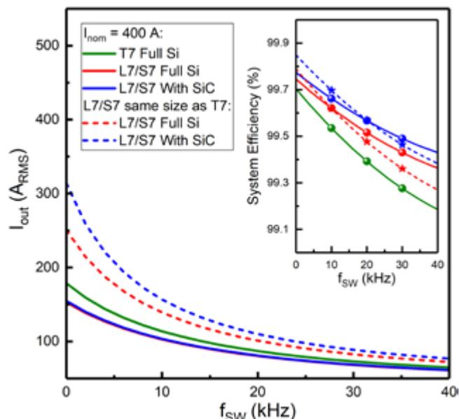
Figure 5:  $I_{out}$  versus  $f_{SW}$  for different variants and power densities at equal thermal boundary conditions. Inset: System efficiency versus  $f_{SW}$  for different variants and power densities at the corresponding  $I_{out}$
