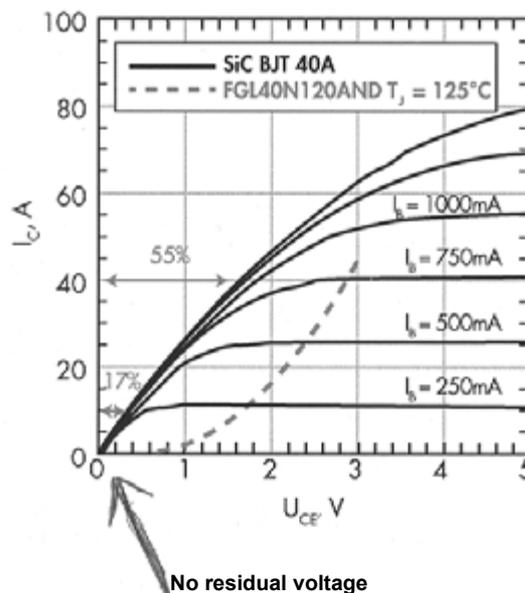
Figure 7.16: Characteristics of the Fairchild SiC BT at 150 C. There is hardly a saturation voltage visible, in contrast to an IGBT. The difference at 40 A is impressive.
