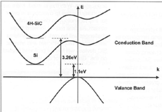
Figure 7.4: The band gaps of Si and SiC. The higher band gap allows high temperature operation at 250 C and kilovolts. SiC takes 10 times higher fields than Si. Theoretically even operating temperatures of > 500 C were possible.
