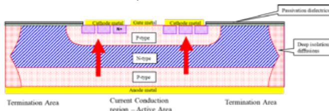
Figure 4: Cross-section of high voltage SCR (both active area and termination areas are shown)
