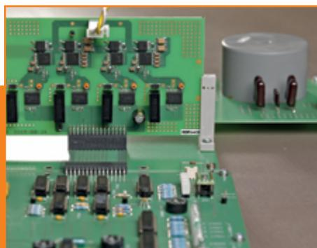
GaN-based output stage for RF surgery applications, with output power up to 150W at 475 kHz. The unique efficiency of the GaN devices enables smaller and quieter surgery equipment.
