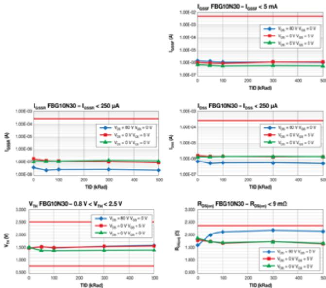
Figure 2: Results of gamma radiation testing of eGaN devices to 500 kRads
