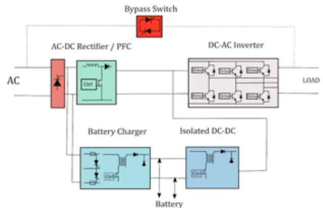
Figure 2: Online UPS topology with high voltage SCRs
