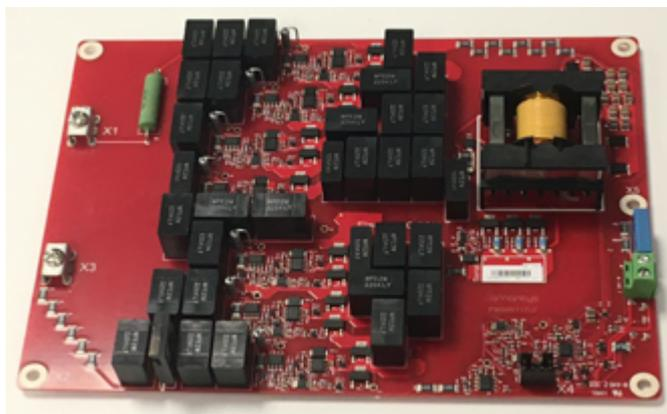
Figure 3: Sub-module Power Supply.
