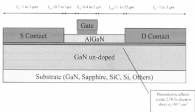
Figure 8.2: Structure of current GaN enhancement transistors.
