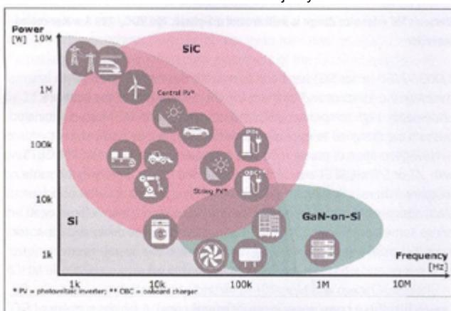
Figure 8.1: Projected application areas for SiC and GaN by Infineon. visualizes that GaN is only applicable to small powers and above 100 KHz. Electric vehicles which require several ten to hundred KW are out of reach for GaN.
