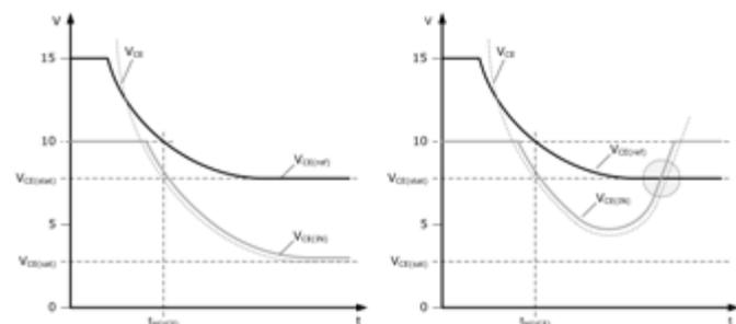
Figure 5: IGBT turn-on behaviour
