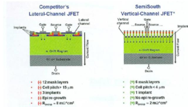
Figure 7.13: Comparison of Semisouth's jfet with that of a competitor.
