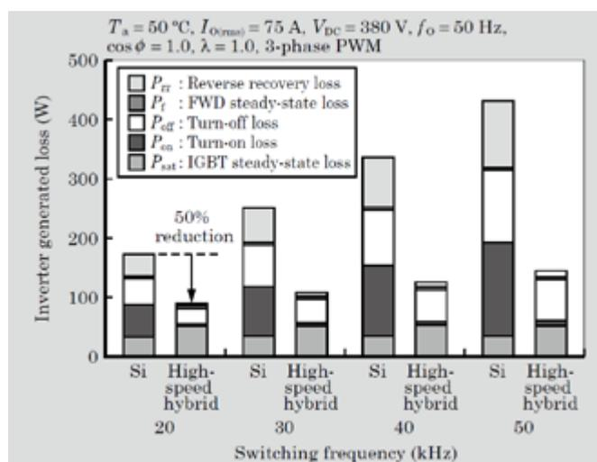
Figure 4: Inverter loss comparison
