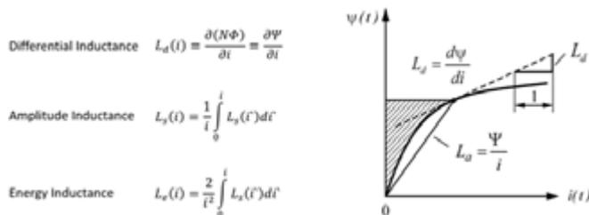
Figure 1: Definition of amplitude inductance, differential inductance and energetic equivalent inductance.
