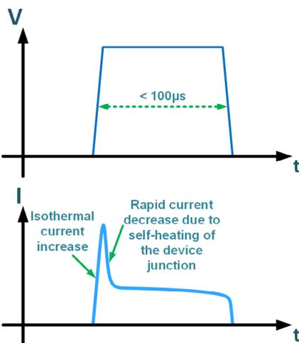
Figure 4: Typical dynamic response of a SiC CLD.
