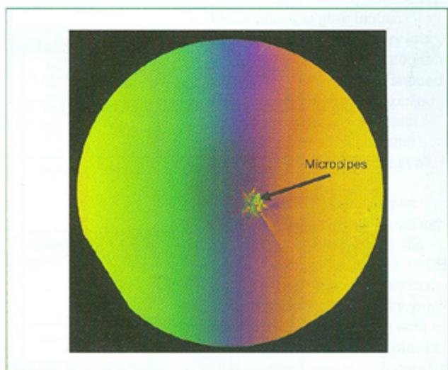
Figure 7.3: The picture shows so-called micropipes which render the material unusable. Those are holes which look like a tornado, they are some micrometers in diameter and go all the way through the whole wafer. For many years they were the main cause of low yield.
