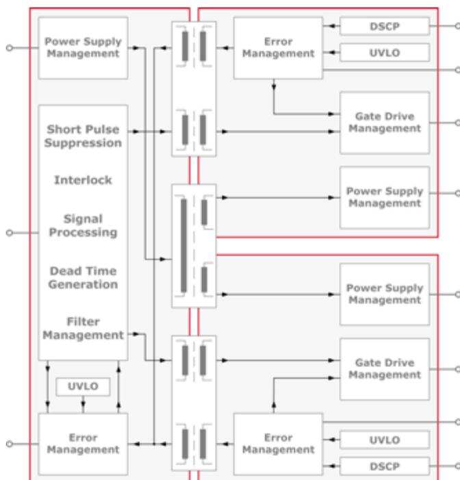
Figure 4: SKYPER driver cores, structured into three major functional blocks
