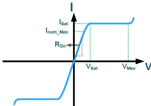
Figure 3: Typical DC behavior of a SiC CLD.
