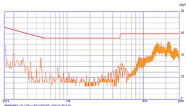
Figure 5: AC-DC power supply with an external filter added
