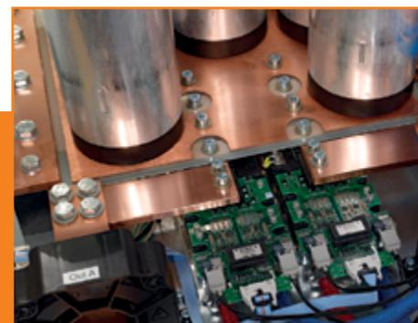
Medium frequency converter module for advanced welding processes in battery cell production for electric vehicles. 4 of these modules in multiphase operation (600 kW output power each) deliver 2.4 MW with negligible ripple current.
