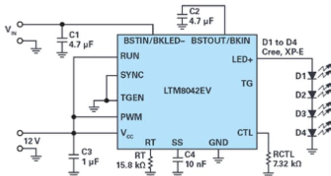
Figure 1: The LTM8042 driving four LEDs where  $V_{IN} = 5.75$  V to 10.25 V and  $I_{OUT} = 0.5$  A.
