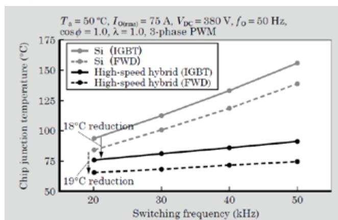
Figure 5: Chip junction temperature when mounted to the inverter
