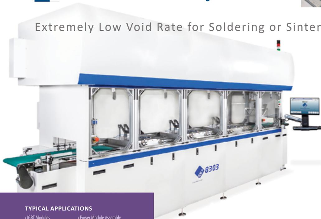
The SST 8300 Series Automated Vacuum Pressure System provides superior bond technology for **soldering or sintering**, plus maximized throughput with a flexible production line development. It is an extremely scalable and module system that allows for upscaling the number of chambers to reach the needed UPH.
