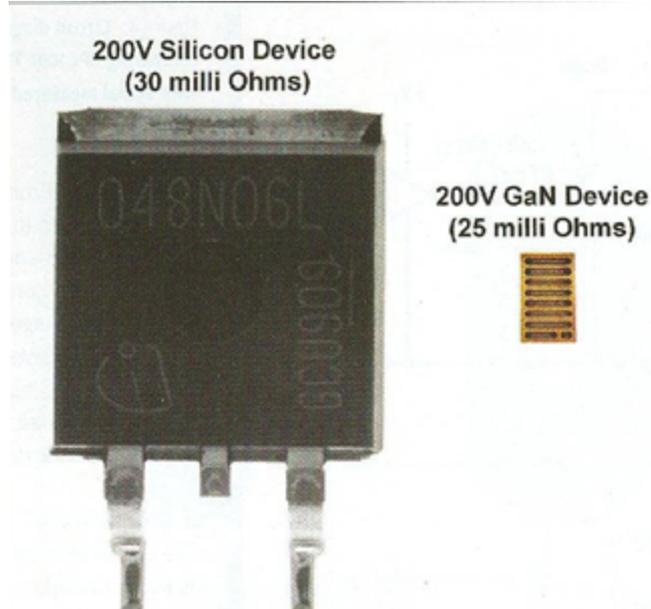
Figure 8.3: Size comparison of a Si and a GaN transistor of identical  $R_{ds(on)}$ .
