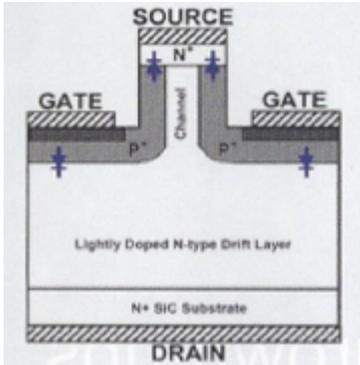
Figure 7.10: Structure of a SiC trench jfet. Like with any jfet there are diodes between gate and channel and drain and channel. At 0 V gate voltage the channel is already fully conducting. If the gate voltage is increased to about 0.6 V, the diode will be on, and the gate input becomes low-impedance. If the drain current is increased the drain potential will rise.
