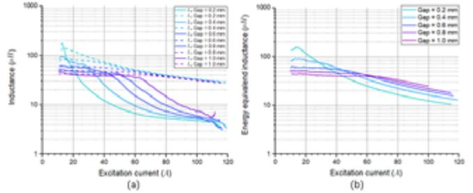
Figure 7: Measurement results for EE65/D9B material ferrite with Bs&T pulse (a) Differential and amplitude inductance (b) energy equivalent inductance
