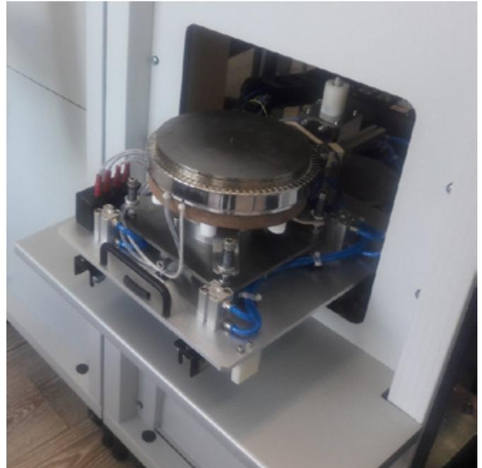
Figure 3: The clamping system with extended draw-out system
