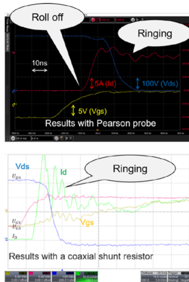
Figure 2: Distorted current measurement results on GaN FET.
