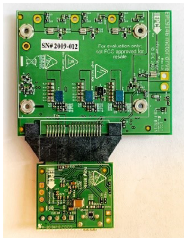
Figure 8: Three-phase BLDC motor drive using EPC2152 monolithic power stages.
