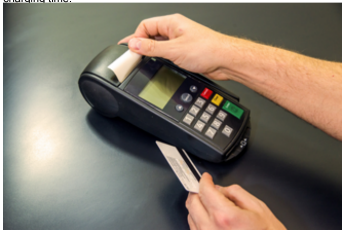
Figure 1: Mobile Point-of-Sale Terminal with a Thermal Printer
