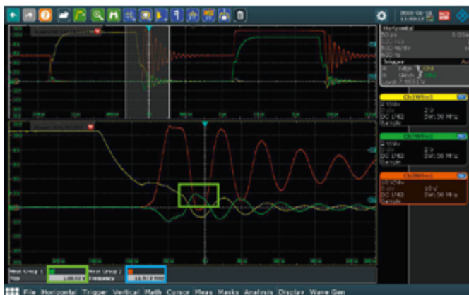
Fig. 3: Measurement result of a half bridge configuration.
