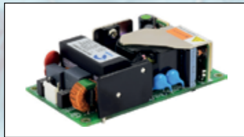
MAD40 open-frame version: 40 Watt on 2" x 3.5" PCB
