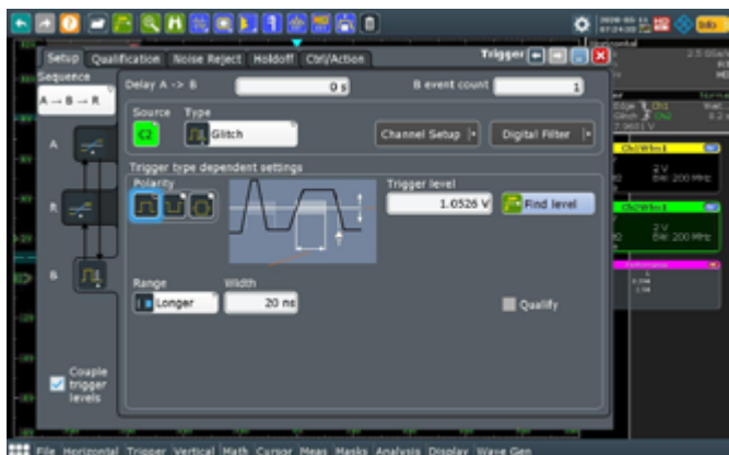
Figure 2: Trigger setup: Glitch event for trigger B at the high-side switch.
