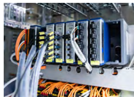
Figure 6: Time-precise control via fiber optic cables and analog measurement
