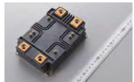
Figure 17: 6.5 kV Full-SiC power module in HV100 package with 10.2 kV insulation voltage
