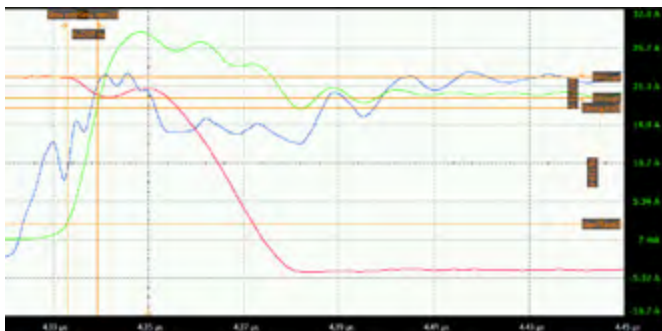
Figure 4 – Parasitic power loop inductance ( L_{PL} = 87.27\text{V}/(16.16\text{A}/6.43\text{ns}) = 35\text{ nH} ) extraction.
