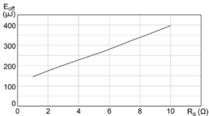
Figure 5: E off vs. R g at VDD=800 V, I D =20 A, VGS=-2 V to 20 V, T j =25 °C as been tested and calculated in [3]
