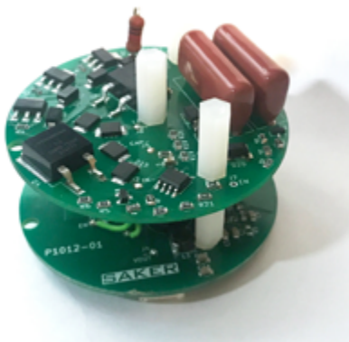
Figure 4: 2.5kV to 5V non-isolated switched power supply prototype, external inductor not shown. Input current is kept in the low mA range
