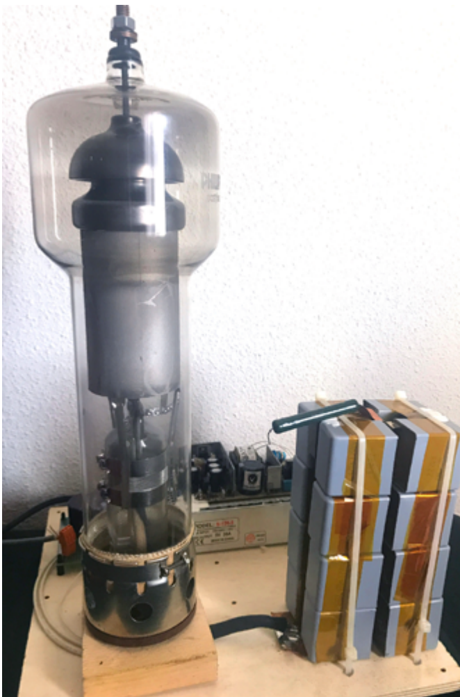
Figure 5: Test setup for a 15kV thyatron.
