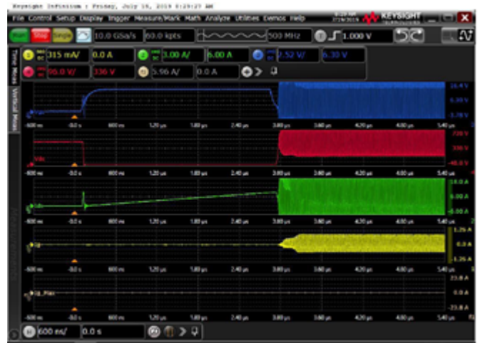
Figure 1: Oscillation at turn off can destroy device and peripheral circuit.
