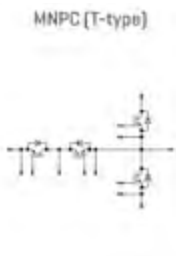
Figure 9: MNPC inverter topology
