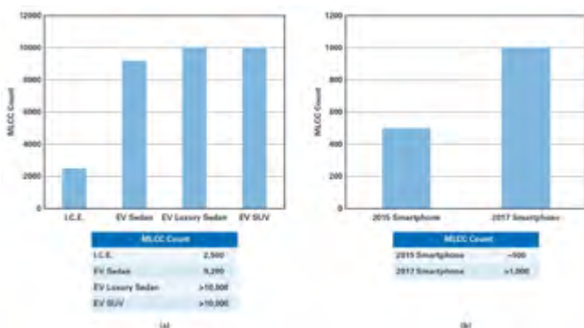
Figure 1: Increases in worldwide MLCC use in electric automobiles (a) and cell phones (b), without commensurate increases in production, have led to shortages. 1
