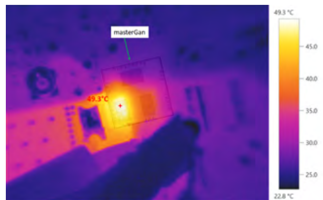
Figure 2: MASTERGAN1 hotspot measured, unknown junction temperature
