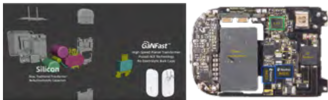
Figure 2: OPPO 50W Mini "Cookie" charger, showing high-frequency planar magnetics and elimination of electrolytic bulk capacitor.
