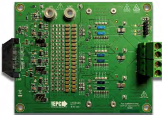
Figure 2: EPC9145 - 3 phase inverter power board based on EPC2206 - 10 x 12 cm
