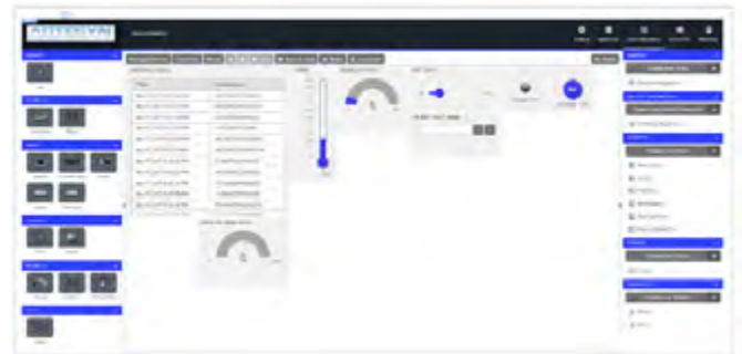
Figure 2: Digital control affords greater levels of scalability, as multiple iHP systems can be controlled simultaneously as routines and power variations can be synced or altered from one cloud-based access point.
