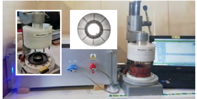
Figure 3: Device Under Test cored with discretely distributed multi gapped (8 gaps/ 0.7 mm for each) toroidal shape, adaptor with defined wire & number, number of turns(10) and its terminals in experimental set up with BsT-pulse micro (with friendly support by Tridelta Weichferrite GmbH)
