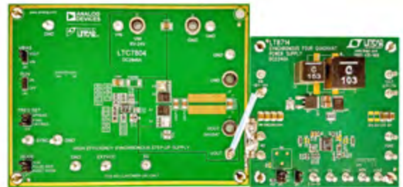
Figure 6: Photo of the test fixture produced by soldering together two off-the-shelf demo boards from ADI. On the left, LTC7804 (DC2846A). On the right, LT8714 (DC2240A).
