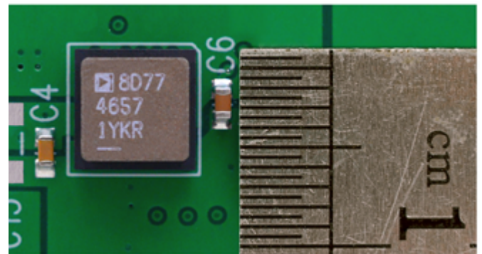
Figure 3: A tiny LTM4657 solution with input and output capacitors on a DC2989A demonstration board. A few ceramic capacitors and a resistor are placed on the back of the board.
