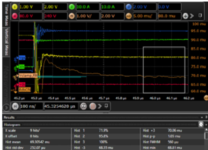
Figure 3: Turn-on switching waveform of a 650 V rating GaN E-HEMT obtained by the newly developed GaN test board with a clamped circuit.
