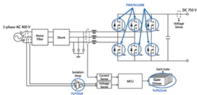
Figure 3: The TW070J120B SiC MOSFETs are coupled with the TLP5214A gate driver in Toshiba’s 3-phase, 400 V PFC reference design.
