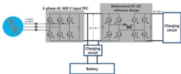
Figure 4: The Toshiba 3-phase, 400 V PFC reference design is ideal for use with bidirectional DC-DC converters in battery charging applications.
