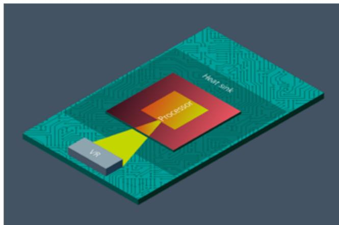
*Figure 1: A typical processor package, shown in red, is 60 x 60mm. All of the current is consumed by the core at the center. PCB resistive losses and parasitic capacitance/inductance in the path to the core are what is called the "last inch" and is the limiting factor to ensuring maximum processor performance.*
