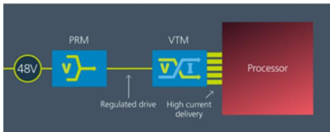
Figure 2: PRM™ and VTM™ are the building blocks of FPA. PRMs are selected based on the system input voltage range and power requirements; VTMs are selected based on the output voltage range and current requirements. The PRM can be mounted anywhere in the system where convenient; the VTM should be mounted as close to the processor core as possible.
