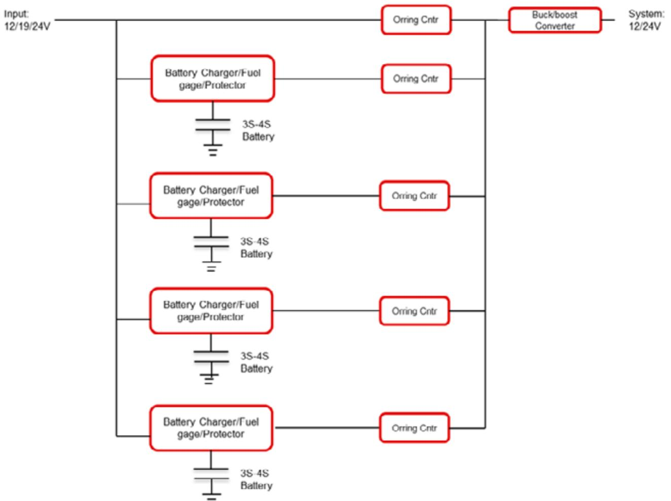
Figure 2: A simplified multi-battery pack battery-management system
