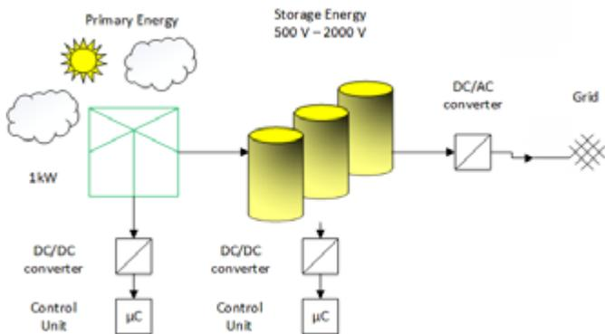
Figure 1: DC/DC converters in application
