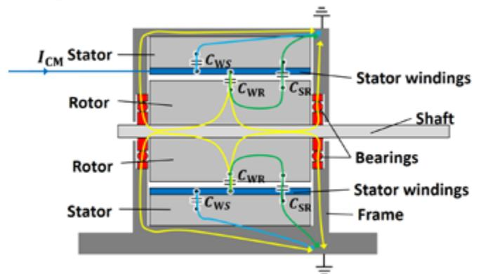
Figure 1: Different current paths for high-frequency CM currents induced to the machine by the converter.
