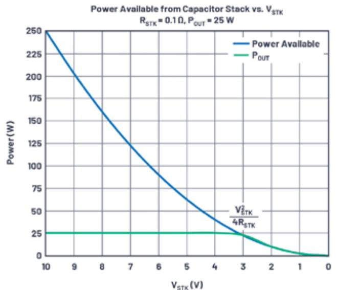
Figure 5: This diagram shows the derivation of minimum  $V_{IN}$  required for certain output power.
