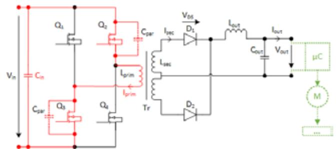
Figure 2: Full-bridge converter topology with midpoint circuit
