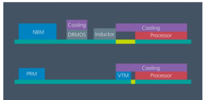
Figure 4: In a typical multiphase VR, the phase inductor height typically limits its proximity to the processor and separate cooling is required for the DRMOS stage. The low profile of the VTM allows it to move under the processor heat sink and associated hardware, while PRM can be placed farther away without loss in performance.
