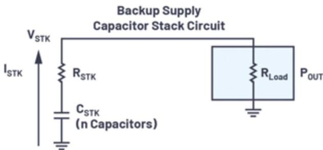
Figure 3: Power delivery from a capacitor stack with series resistance.
