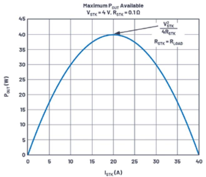
Figure 4: Curve of available power vs. stack current.
