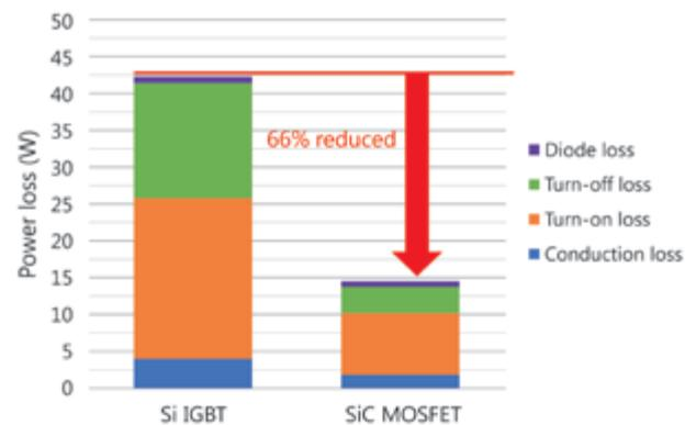
Figure 2: Implemented in a 3-phase PFC, the SiC MOSFET shows a 66% reduction in power loss compared to an IGBT-based design.
