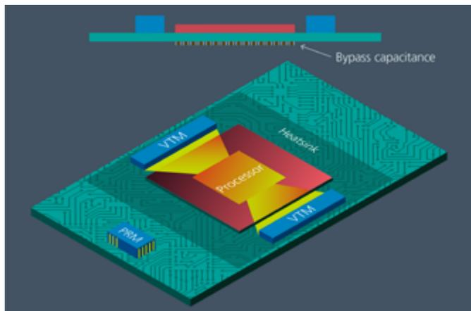
Figure 3: Typical PRM/VTM Factorized Power Architecture solution supporting main rail power on an AI accelerator card. Placing VTMs on opposite sides of the socket divides current flowing through the power delivery network to the processor in half and reduces losses by 50%.
