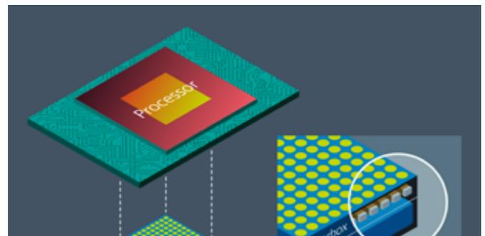
Figure 5: Vertical power delivery (VPD) with GTM Geared Current Multiplier placed underneath processor maximizing power delivery performance. The VPD solution also relieves the processor top-side periphery for options including higher I/O routing, onboard memory, or tighter processor clustering.
