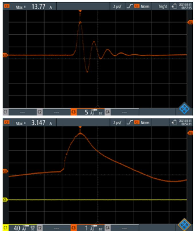
Figure 5: Typical CM-current pulse pattern without counter measures (upper screen) and after the injection of current chokes (lower screen)
