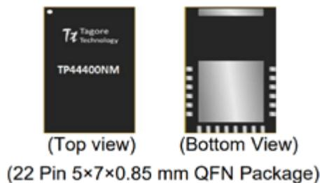
Figure 1: Tagore 360mΩ GaN Power IC, TP44400NM
