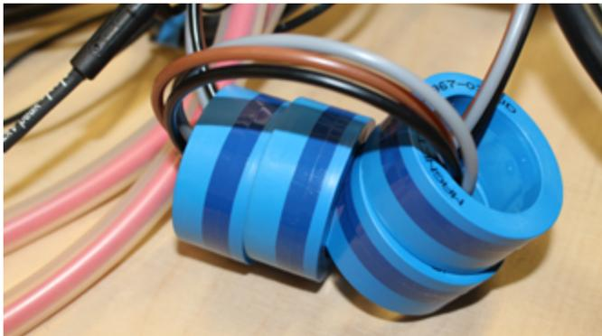
Figure 4: Four high-permeability ring cores are connected in series as current compensated chokes with 2 windings in total.
