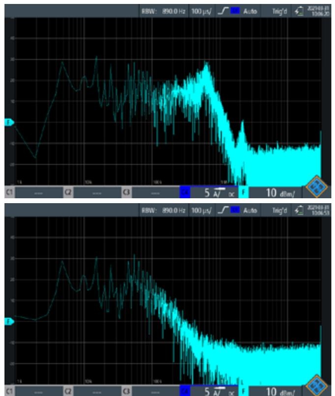
Figure 6: Visualization of the frequency of the CM current using the FFT-function of the oscilloscope. The spectrum before the insertion of the chokes is shown on the left, the spectrum after the insertion is shown on the right side.
