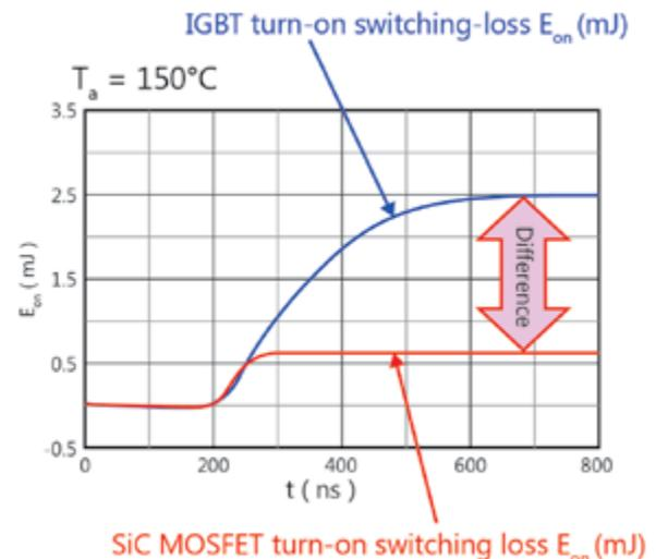
Figure 1: Compared to latest-generation IGBTs, the TW070J120B SiC MOSFET shows considerably faster switching speeds that deliver higher efficiencies in power converters.
