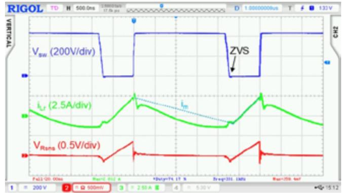
Figure 3: GaN drain switching waveforms of the QRF (left) and ACF (right) chargers.
