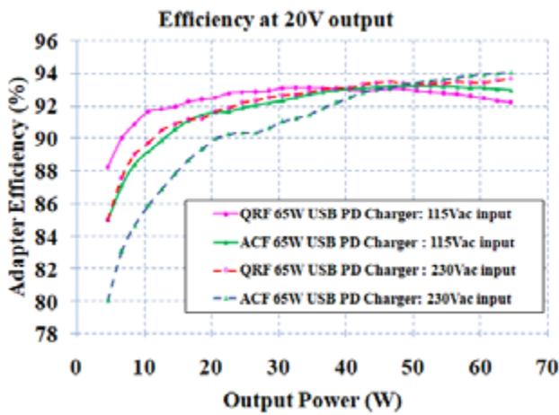
Figure 4: Comparative efficiencies of QRF and ACF chargers.
