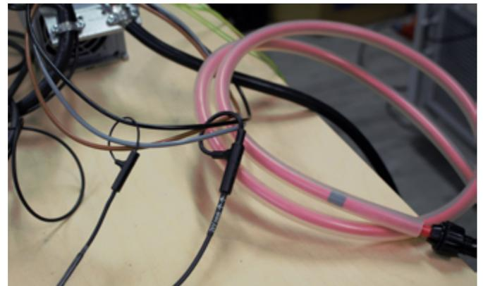
Figure 2: Measurement of CM current with three different Rogowski coils from PEM UK [8] - left: PEM CWT Ultra mini, middle: PEM CWT miniHF, right: PEM custom made (2 windings)
