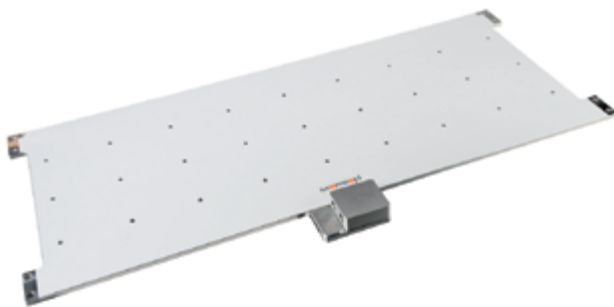
Figure 6: Mersen offers flexible cooling solutions – the picture shows a 7mm thick AL vacuum brazed liquid cold plate for battery cooling. Image © Mersen
