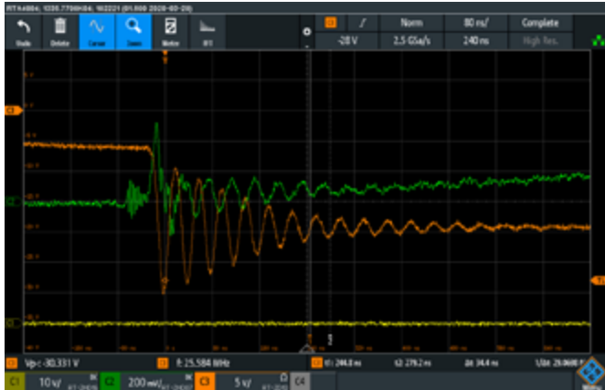
Figure 4: A measured switching diode waveform with no snubber
