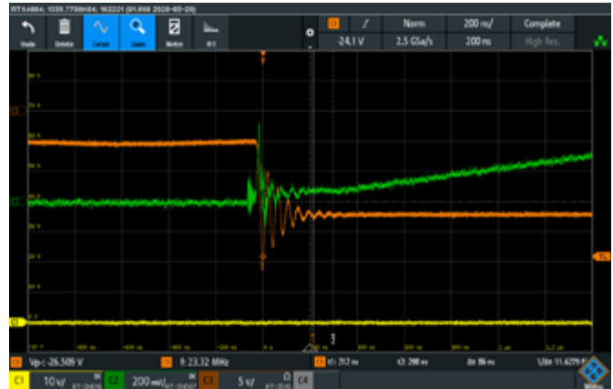
Figure 6: Waveform with calculated snubber values
