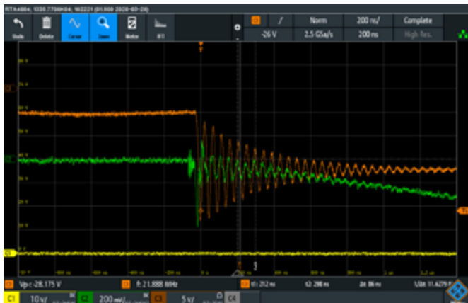
Figure 5: As Figure 4 but with known 178pF capacitor added
