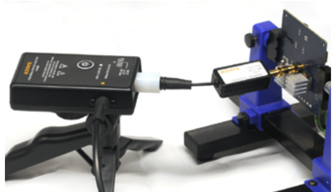
Figure 5: ISOVP connected to the Infineon GaN eval board. Note the direct coaxial connection.
