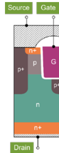
Figure 1: Sketch of the Infineon CoolSiC MOSFET cell structure
