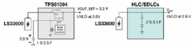
Figure 3: TPS61094 vs. HLC/EDLC configuration
