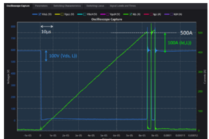
Figure 1: More than 500 A I_d test results on SiC power module (FF2MR12KM1P).
