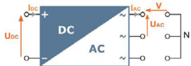
Figure 8: Electrical operating parameters of 3-phase DC/AC converter topology
