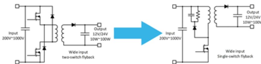
Figure 1: The ubiquitous auxiliary power supply is shown above, using the wide input single-switch flyback topology.
