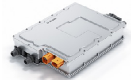
Figure 1: 7-11kW OBC + 2.4kW/14V DCDC presented by BOSCH Mobility Solutions [2]
