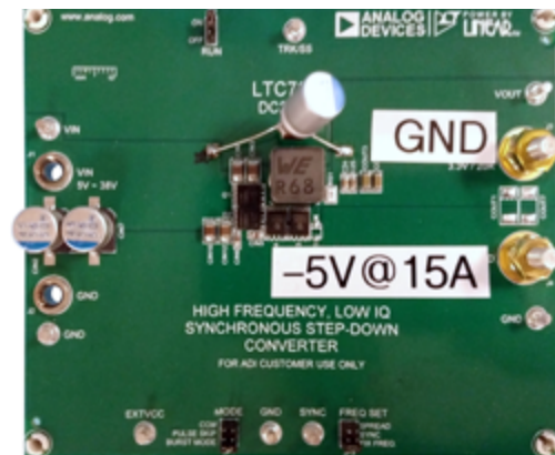
Figure 5: DC2834A converted to inverting buck-boost from the original, off-the-shelf step-down converter.
