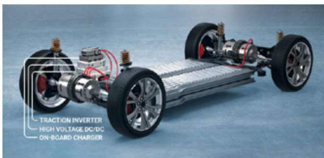
Figure 1: The EV powertrain, including: traction inverter, high-voltage DC/DC, and onboard charger
