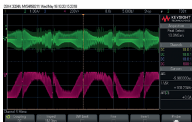
Figure 7: Common-mode interference current (green) and common-mode interference voltage (red) in a PFC converter at a full load of 1000W and a mains voltage of 230VAC
