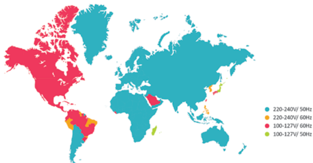
Figure 1: worldwide AC mains single phase voltage and frequency levels without tolerances
