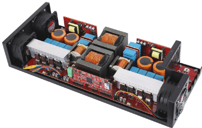
Figure 12: The Infineon REF-DAB11KIZSICSYS reference design board has an 11 kW output rating
