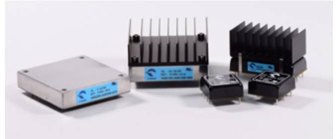
Figure 8: All P-duke modules come in a robust silicone potted housing and cooling can be done either through the baseplate (>100 W) or top of the module (10 – 60 W).
