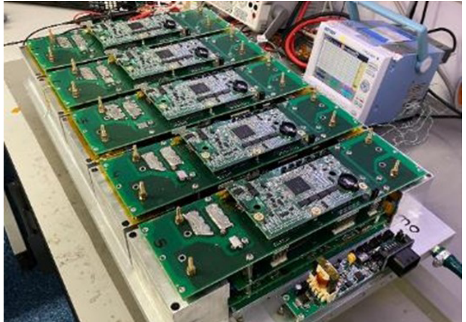
Figure 4: RECOM's Modular 5x15kW (75kW) Fuel Cell DC-DC Converter
