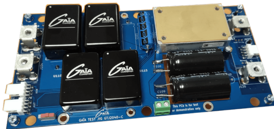
Figure 9: Example of a 250 W power architecture that can be built using evaluation boards, which are fully documented within the "evaluation board service manual" [3.2].
